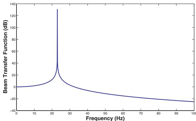
FIG. 3. (Color) Beam transfer function during physics defined by  $[1 \ 0](2\pi ifI - A)^{-1}[0 \ \omega_s^2]^T$ . As expected, the resonance is at the synchrotron frequency of about 22 Hz for the physics configuration. The resonance is even sharper during injection due to the longer synchrotron radiation damping time.
