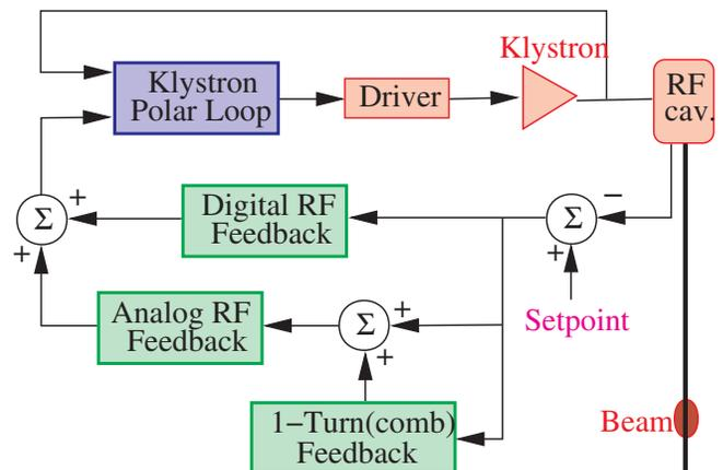
FIG. 1. (Color) Simplified LHC rf block diagram.
