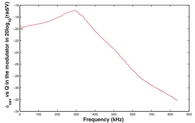
FIG. 4. (Color) The transfer function between the rf accelerating voltage phase and the noise at the  $q$  channel at the input of the modulator  $\{[\phi_{\text{cav}}(f)]/[n_q^{\text{mod}}(f)]\}$  (rad/V).
