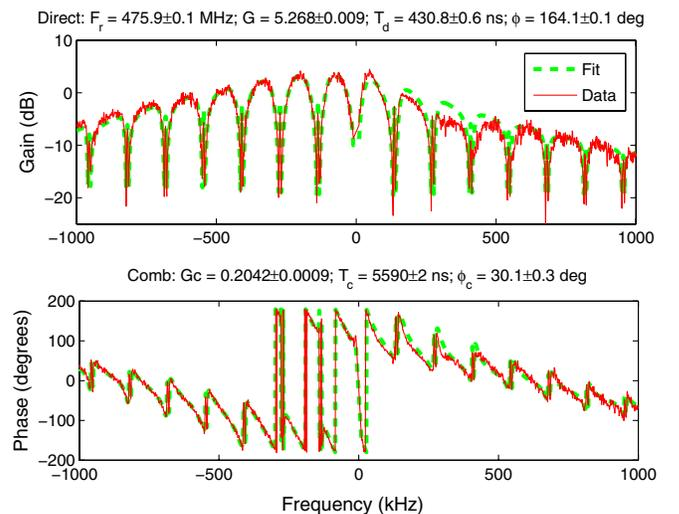
FIG. 3. (Color) Transfer function and parameters of operating station in LER at 1400 mA.
