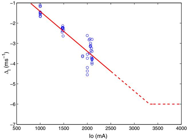
FIG. 7. (Color) Plot of  $\Delta_1$  with current in mA. The  $-6 \text{ ms}^{-1}$  limit is from the low-mode longitudinal control path.
