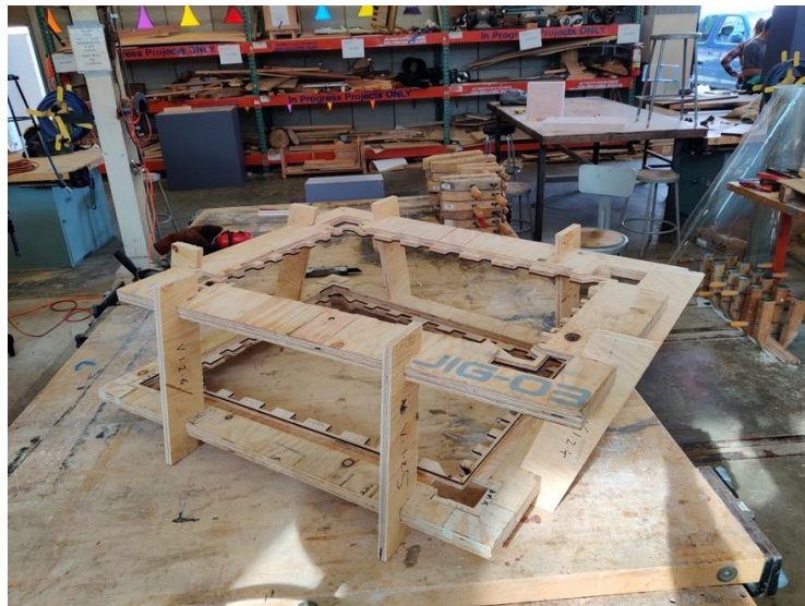
Figure 3: Fully constructed jig
