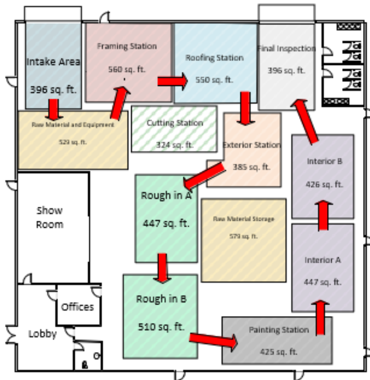
Figure 4. Floor Plan Layout of Production Line Facility
