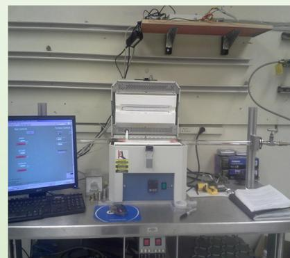
Figure 3. Furnace used for CVD
