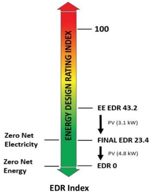
Figure 1. Energy Design Rating (EDR) Index Example (Lieu, 2019)
