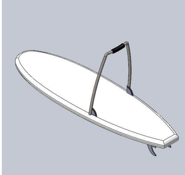
Figure 22.1 Preliminary model of folding standing support in upright position.
