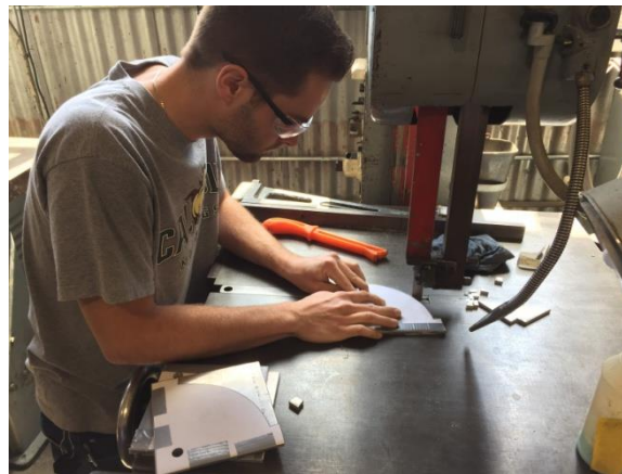
Figure 30. The team initially used a vertical band saw to rough cut the round edge of the guide plates.
