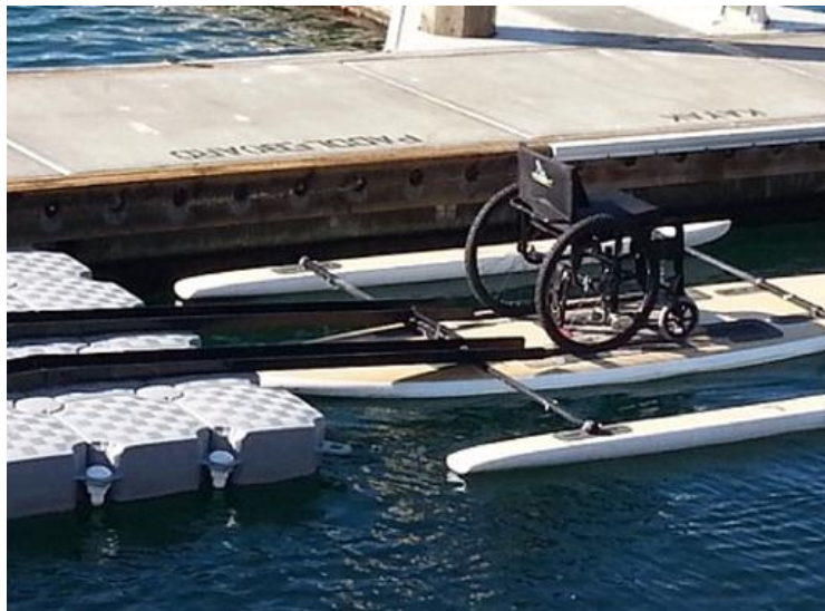
Figure 7. The Onit Ability Board with a wheelchair locked in and the aluminum ramp for user boarding. [6]
