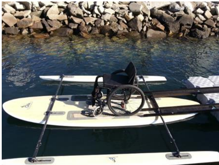
Figure 8. The Onit Ability Board shown clearly with its two outriggers. [6]
