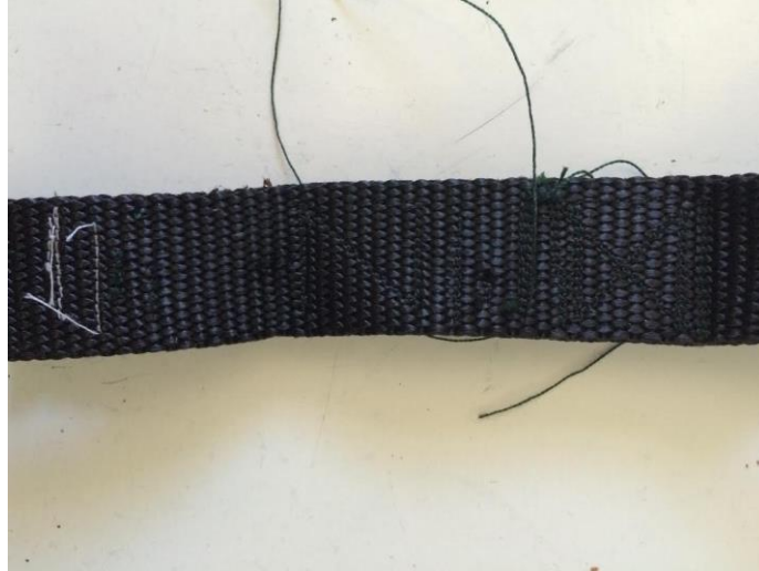
Figure 40. Failed stitching patterns and thread in nylon straps.
