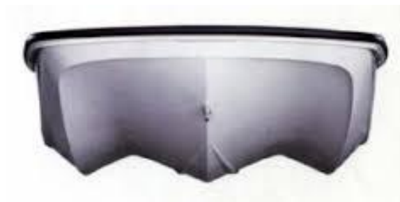
Figure 10. Front view of a cathedral hull of a boat. [7]
