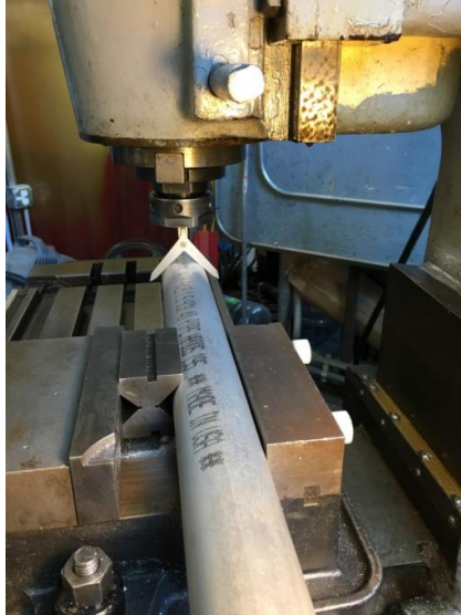
Figure 31. The centerline of the vertical supports were found to ensure the accuracy of milling operations.
