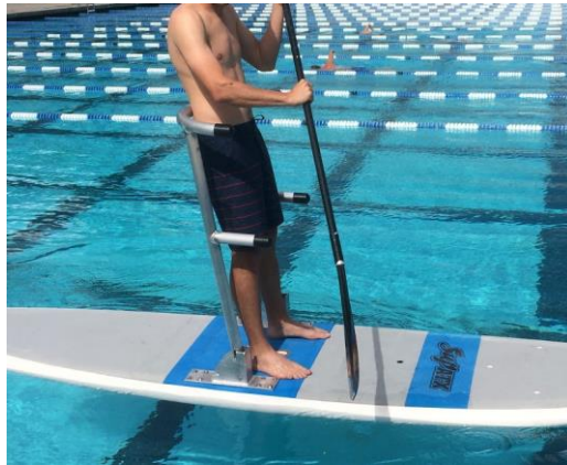
Figure 36. Loading of the support structure at the furthest moment arm from the joint to check for joint integrity.
