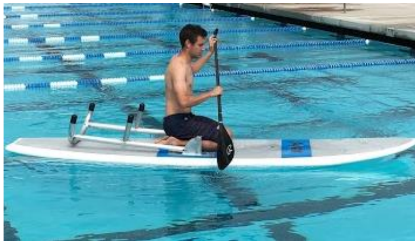
Figure 37. During testing at the Cal Poly Recreation Center pool, a variety of users rode the board in each of the multiple riding positions for a prolonged period of time to test the board's ergonomic features.
