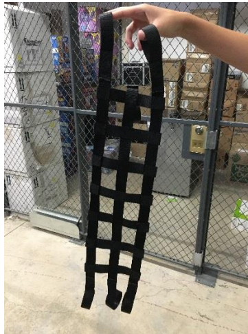
Figure 33. The nylon webbing seat that was selected instead of a full-fabric design.
