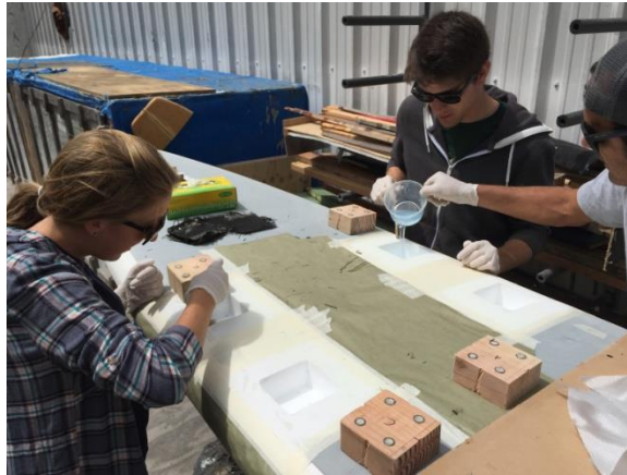
Figure 28. Epoxy resin being applied to the bottom layers of the “top hat” lay up before the wooden inserts are positioned.
