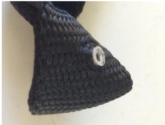
Figure 39. Failed rivet in the nylon strap that was to be used for the seat.
