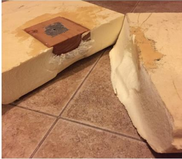
Figure 38. The results of the surfboard blank and wooden insert test, which shows the torn foam and intact wooden insert after loading 120 pounds onto the test rig.
