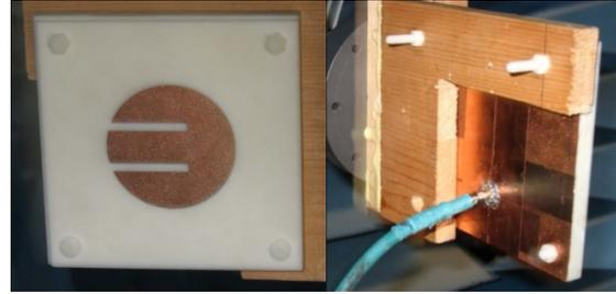
Fig. 5. Fabricated Circular-E Patch Antenna.
