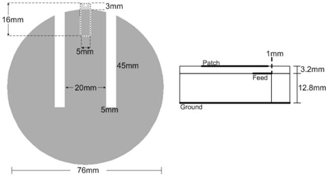
Fig. 3. Circular-E Patch [3] Optimized Dimensions.
