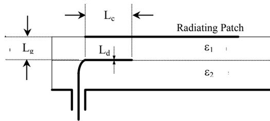
Fig. 4. Microstrip L-Probe Antenna Feed.
