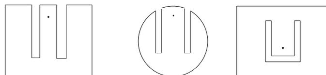
(a) Rectangular E-shaped Patch (b) Circular E-shaped Patch (c) U-shaped Slot Patch
