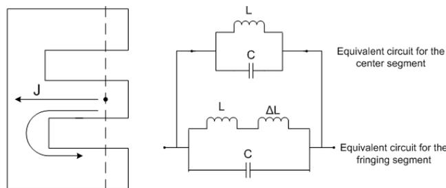
Fig. 2. Microstrip Patch Antenna Equivalent Circuit.
