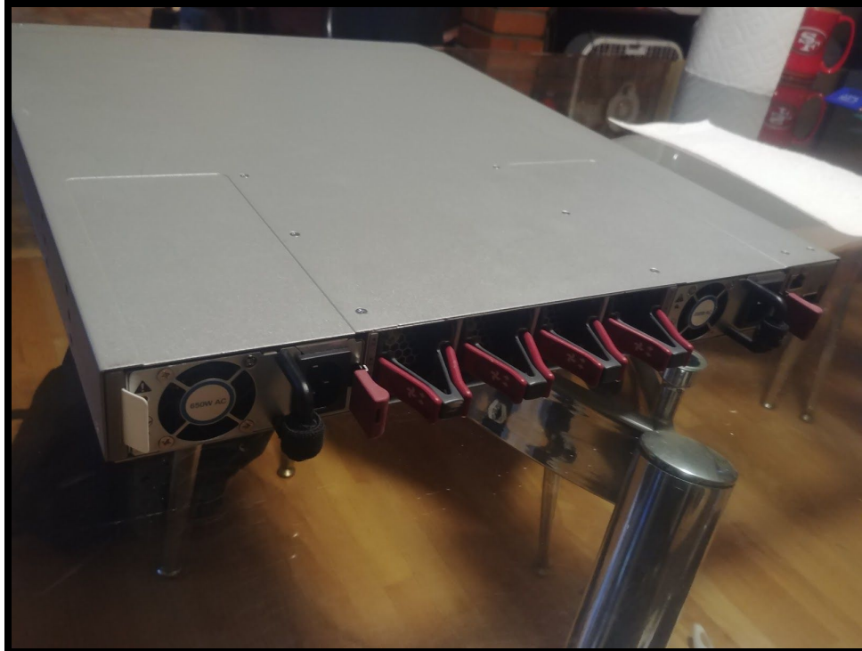
Figure 7: Rear View of Physical Nexus 9200 Chassis
