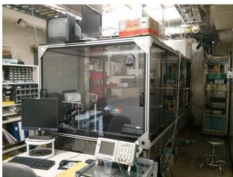
In order to do this, an interferometer has been set up to measure transverse coherence in terms of visibility.
