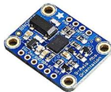
*Figure 6 - Adafruit BNO055 IMU [5]*
