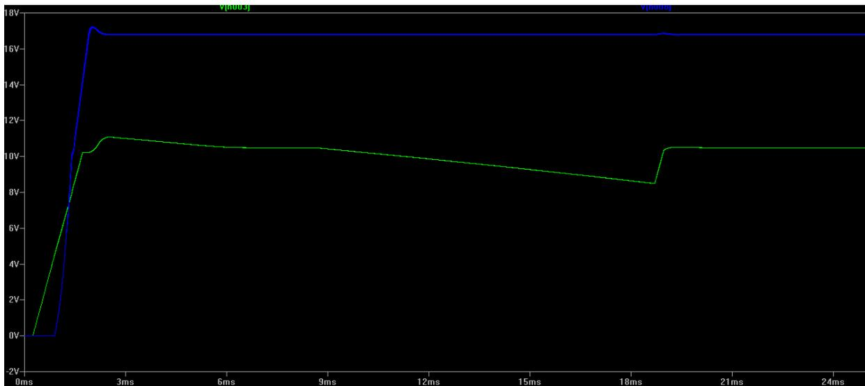
**Figure 4: Simulation waveforms for Buck/Boost Converter. Green=Input, Blue=Output**
