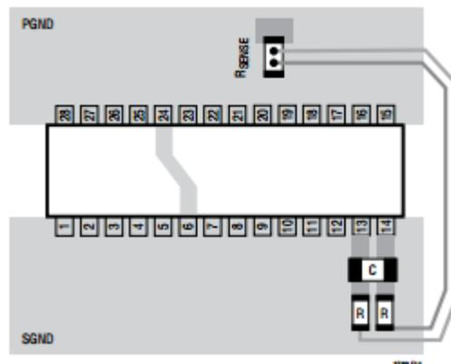
**Figure 8: Suggested layout of Sense Lines [2]**
