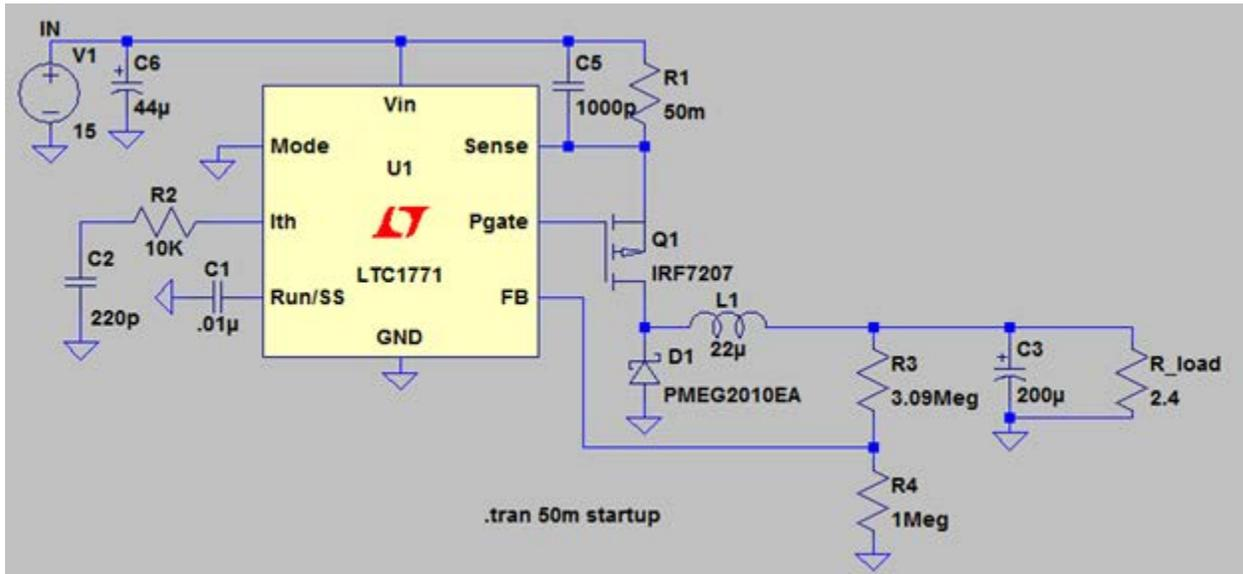
**Figure 9: General Schematic for the LTC1771[3]**
