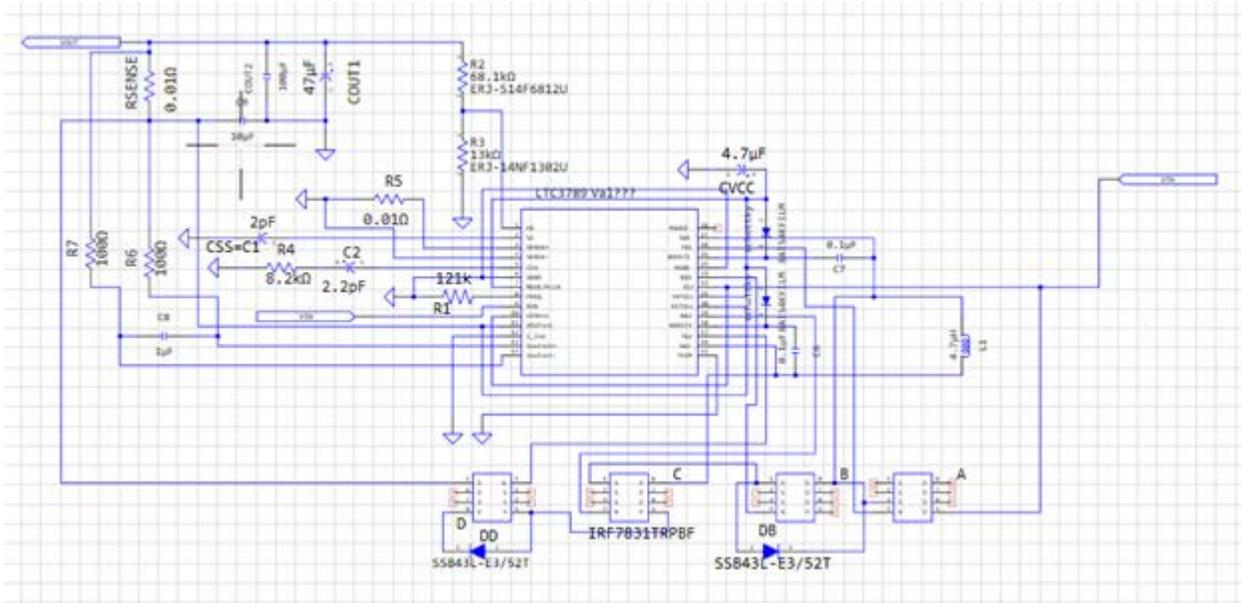
Figure 6: Schematic of Buck/Boost Converter
