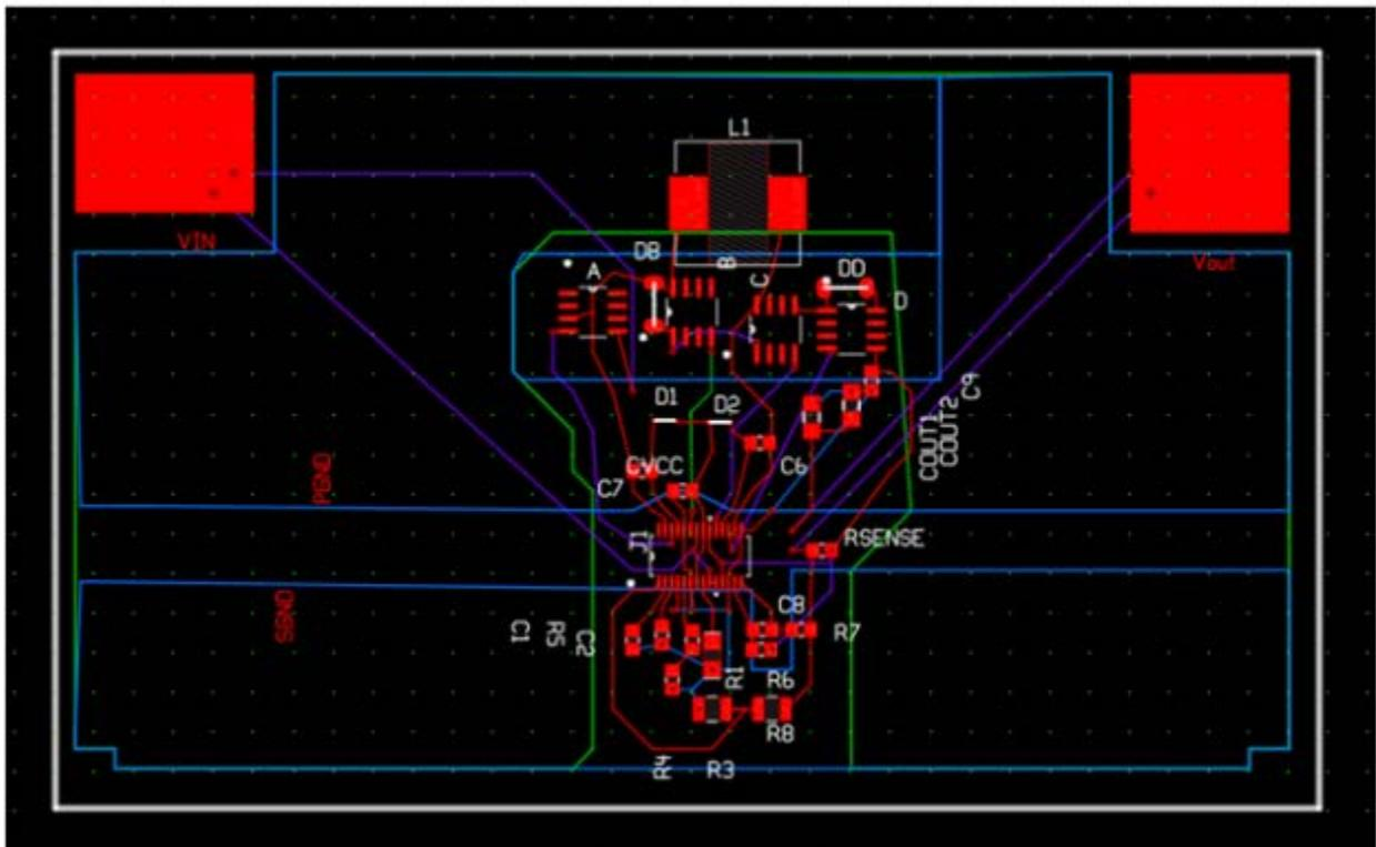
Figure 7: PCB Layout for the Buck/Boost Converter
