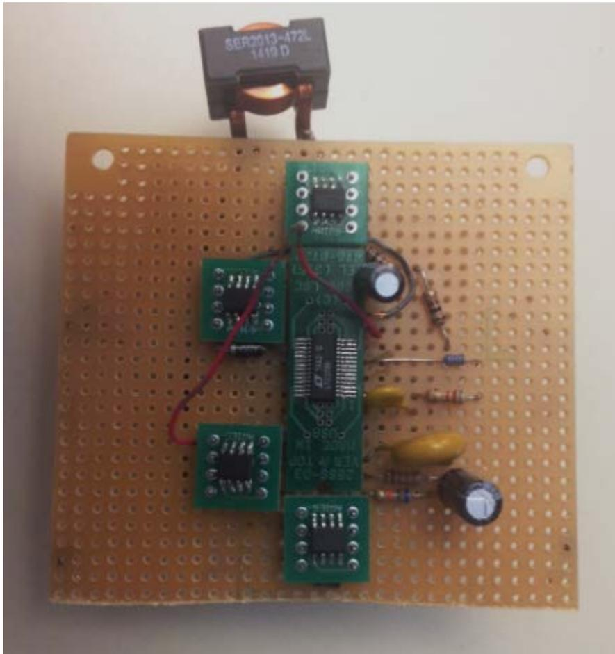
**Figure 5: Design 2 for Buck/Boost Converter**
