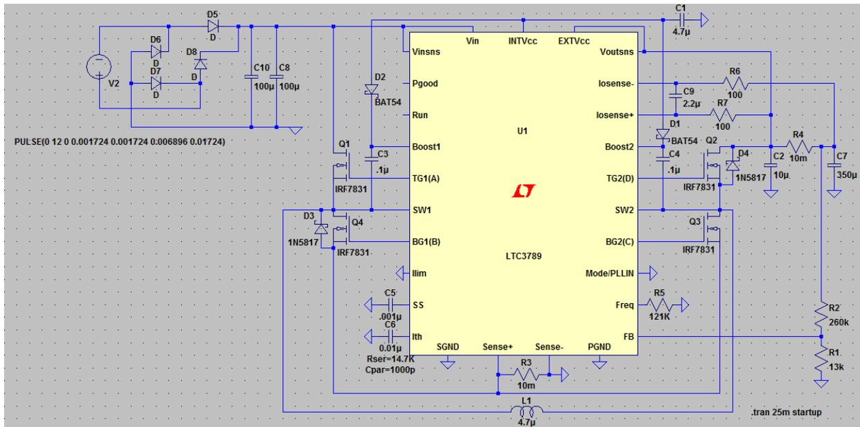
**Figure 3: General Schematic for the LTC3789 [2]**
