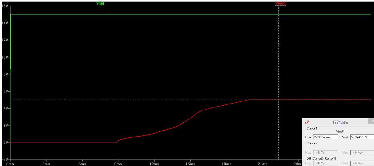
**Figure 10: Simulation Waveforms, Buck Converter (Input = Green, Out = Red)**
