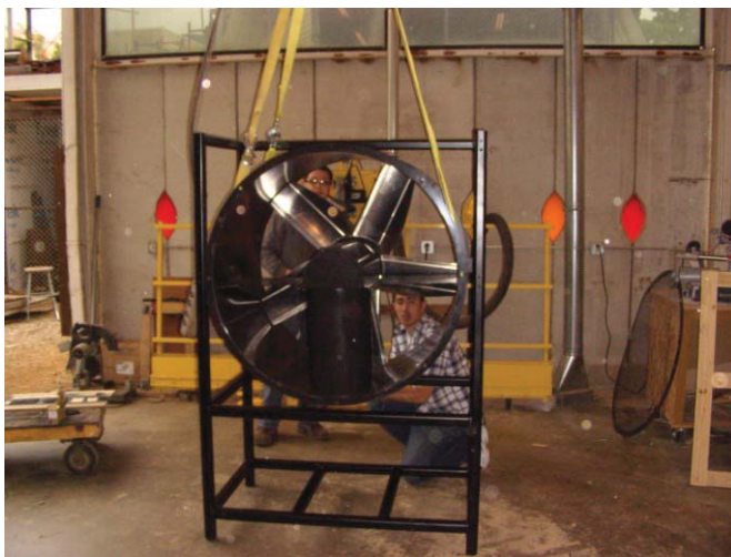
Figure 8. Installation of fan in motor stand.
