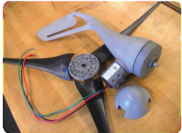
Figure 4. SunForce 400W Wind Generator. Peak output achieved at 28mph wind speed.
