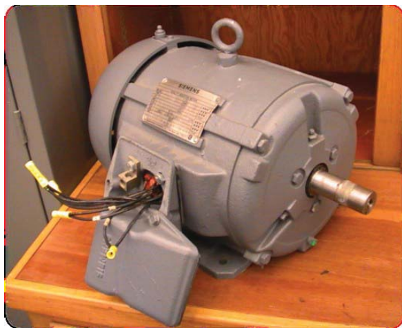
Figure 2. Siemens 3 phase induction motor: 5hp, 13.4/6.7 Amp, 230/460 V, 1740 rpm, NEMA B design, Frame 184T.
