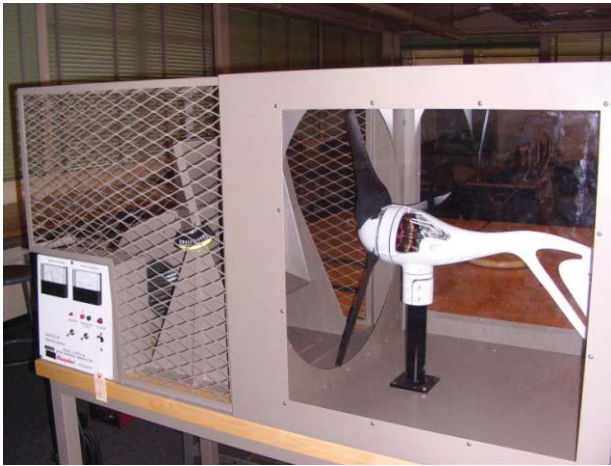
Figure 11. The wind turbine in a wind tunnel chamber
