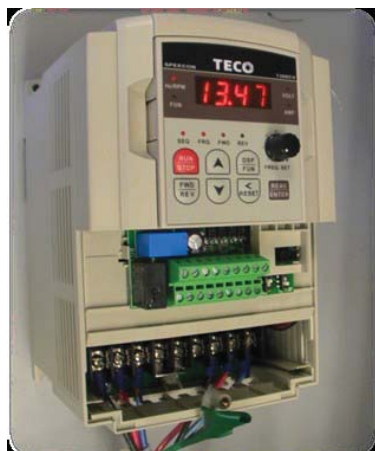
Figure 3. TECO Variable Frequency Drive, 5hp/3.7kW, Input: 3-Phase, 200-240V, 20.5A, Output: 3 phase 0-400Hz, 0-240V, 17.5 A
