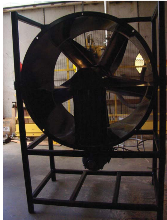
Figure 9. Completed nstallation of fan in motor stans
