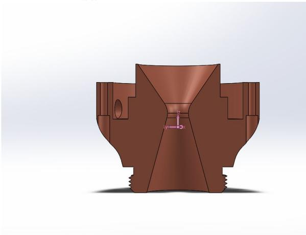
**Figure 5-4** Section view of copper nozzle
