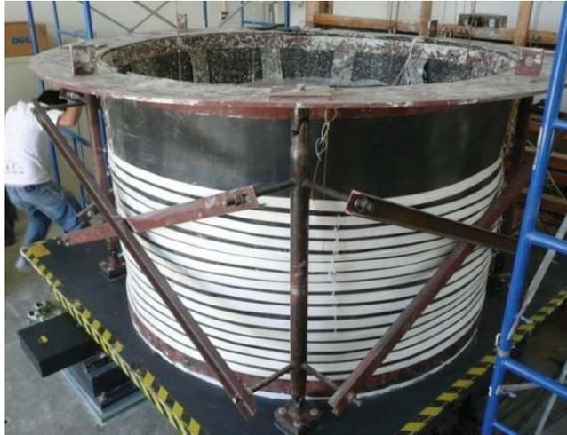
The main testing equipment is a flexible wall barrel that mimics free field site response under seismic loading on the shake table. The flexible wall barrel has been validated through table testing and 1-D equivalent linear numerical analysis in a recently completed research project (Crosariol, 2010; Moss et al., 2010).
