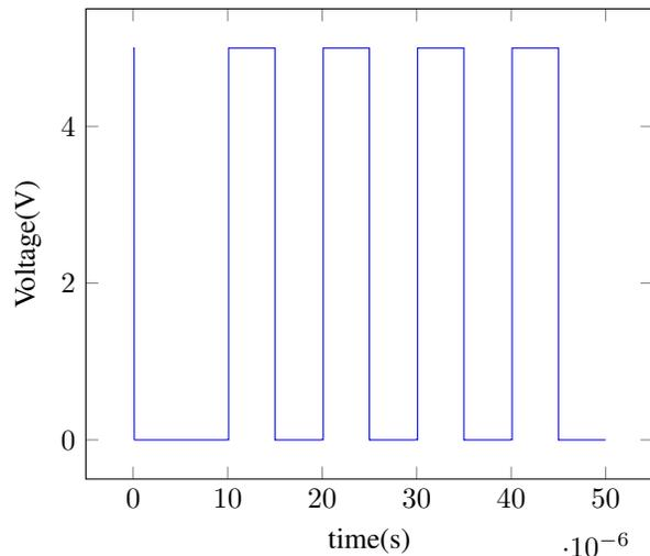
Fig. 4. Functional Output for 2.5 Volt Input. The pulse width of the PWM signal accounts for a large portion of the interval between reset pulses, giving the PWM signal an approximate 50% duty cycle.
