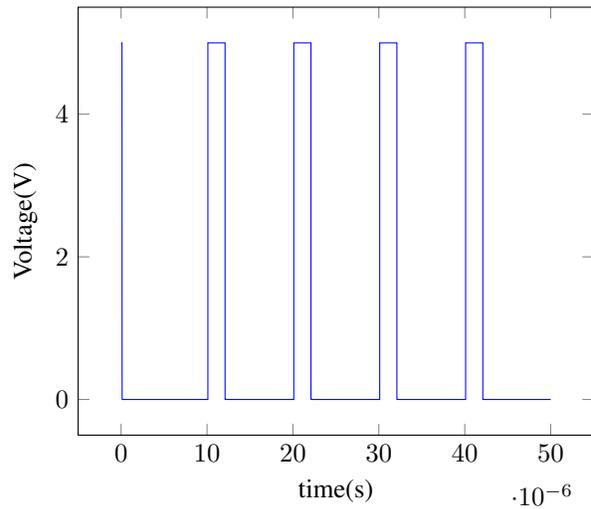
Fig. 3. Functional Output for 1 Volt Input. The pulse width of the PWM signal is slightly larger than in Figure 2, but still relatively small.
