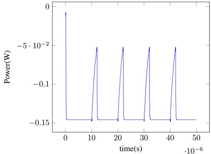
Fig. 8. Power Data for 1 Volt Input. The passive power consumption is about 10x less than in Figure 7, and the active power spikes are less pronounced.
