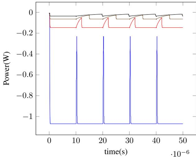
Fig. 6. Initial Design Power Comparison Graph. The power comparison shows that both the active and passive power consumption of the circuit rises as the applied analog voltage decreases.
