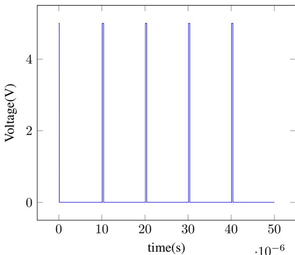
Fig. 2. Functional Output for 0.1 Volt Input. The pulse width of the PWM signal is almost as small as the reset pulse sent to the circuit.
