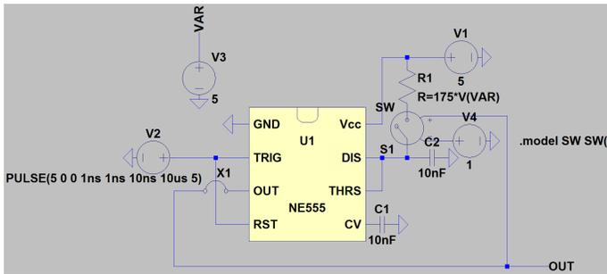
Fig. 1. Schematic for the final version of the PWM generator circuit.
