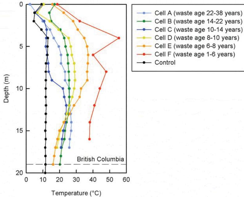
Fig. 3. Temperature Profiles for Variable Waste Age
