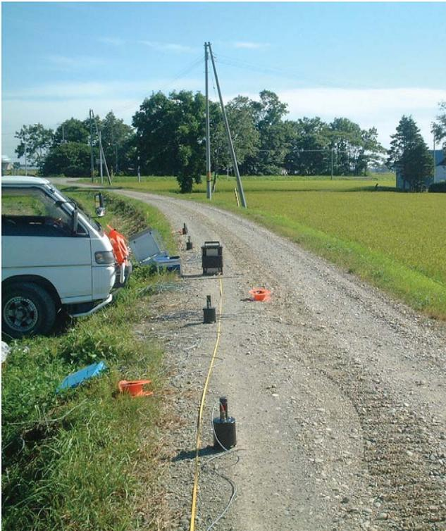
**Fig. 3.** Typical SASW configuration using the portable frequency-controlled, 100-kg electromechanical shaker (center unit) with forward and reverse arrays of 1-Hz sensors (Site 41NAGA, Naganuma, Hokkaido liquefied during the Tokachi-oki 1968 earthquake and not liquefied by the Tokachi-oki 2003 earthquake); Photo by Robert Kayen
