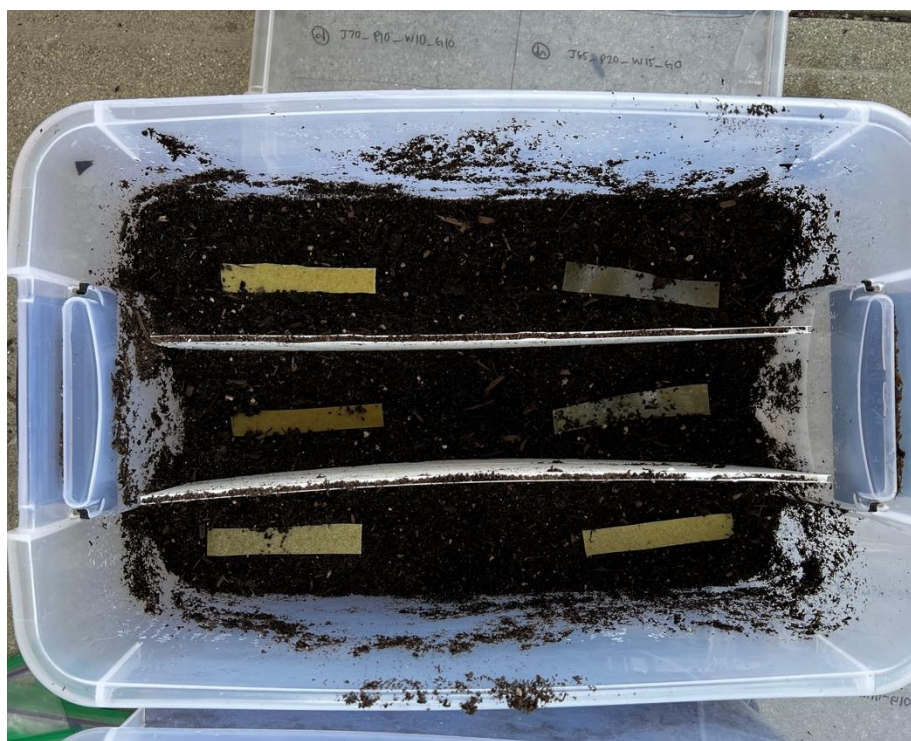
Figure 6. Soil degradation testing bins
