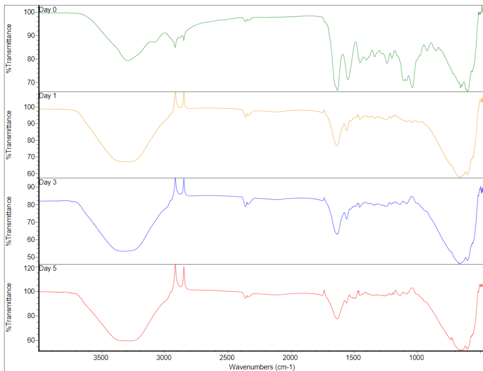
Figure 38 FTIR Overlays, Composition 4
