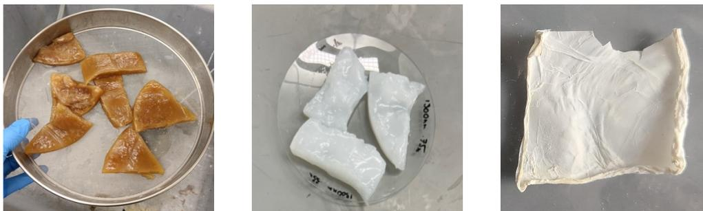
**Figure 6.** BC samples throughout the preparation process: (a) unpurified but fully grown BC samples, (b) BC samples after purification, and (c) a soaked and dried BC/silica nanocomposite sample.
