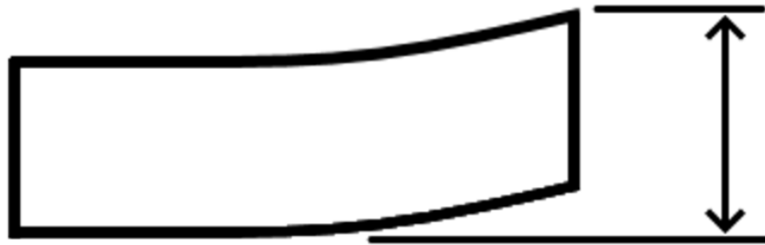
Figure 9: Representative diagram of setup used to measure the degree of sample warping
