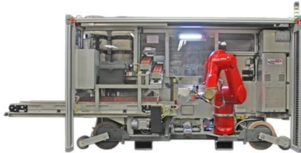
Figure 3: The SAM100 bricklaying robot
