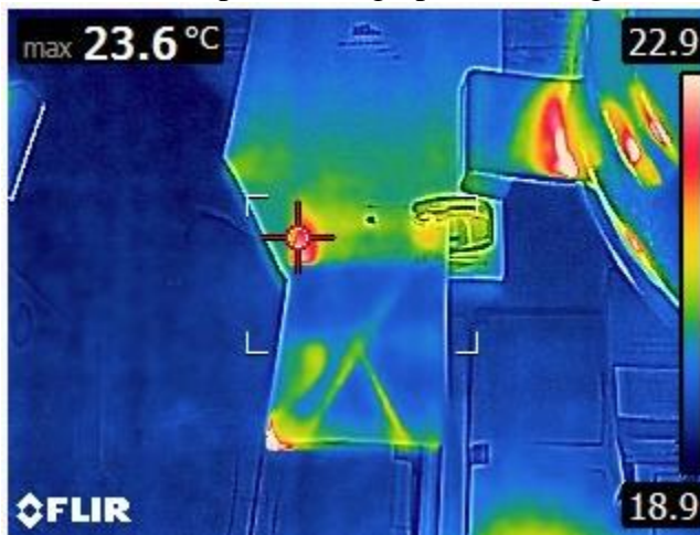
Aluminum sample thermographs and ImageJ images at 0.5 m.
