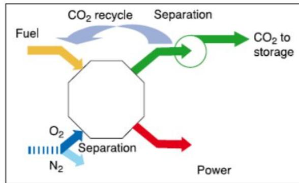
*Figure 3: Schematic of Oxyfuel Combustion*
