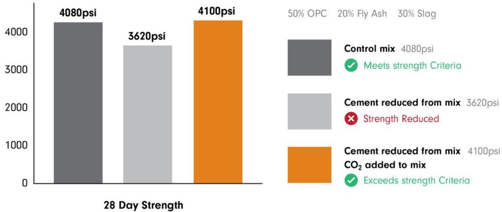
Figure 5: Effectiveness of CO<sub>2</sub> as a Cement Replacement
