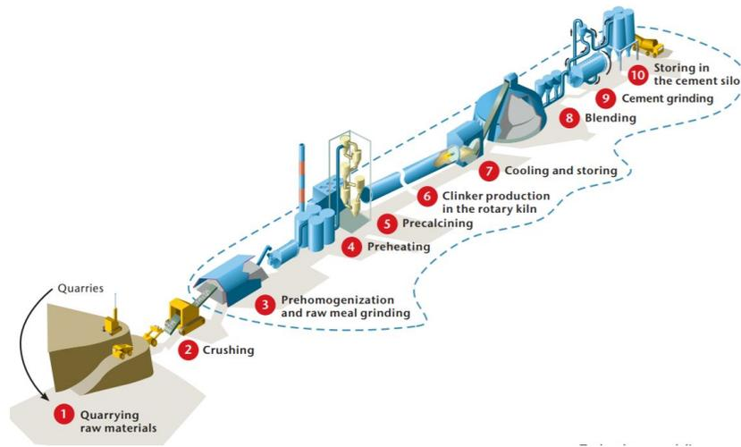
*Figure 1: Cement Manufacturing Process*
