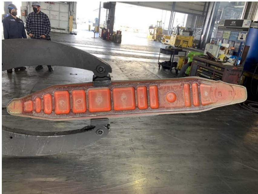
Figure 1: A titanium landing gear beam made of Ti-6Al-4V, manufactured by Weber Metals.
