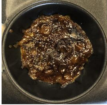
Figure 15. The burnt upper surface of PET in a well after 20 minutes of exposure to 260 °C.
