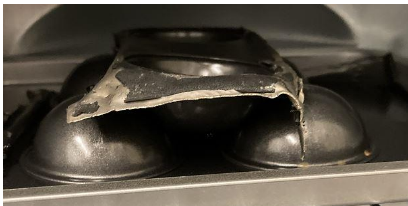
Figure 8. Melt extrusion setup with a 2 well x 1 well pan with 1.75 mm holes drilled in the bottom, placed on an inverted 2 well x 2 well pan.
