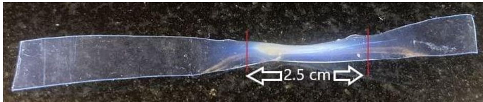
Figure 12. Deformed PET strip after 20 minutes at 95 °C. The area between red lines is the rolled region.
