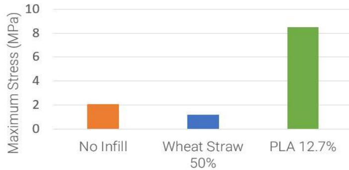
Figure 17. Maximum stress before failure on 50 mm x 50 mm x 25 mm PLA frame with various infills.
