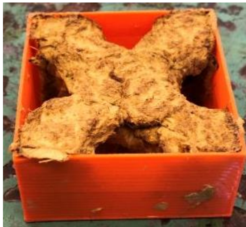
Figure 10. PLA frame with approximately 50% wheat straw infill.
