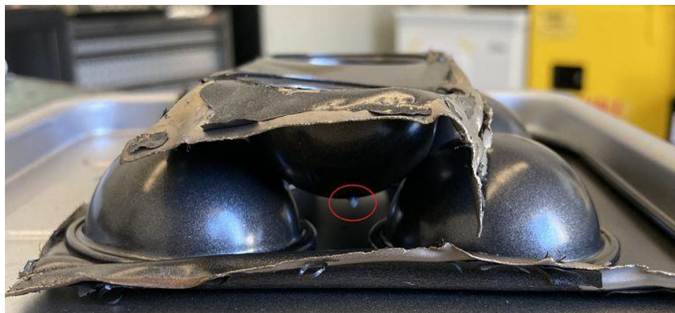
Figure 14. A small length of PET (circled in red) extruded from the 1.75 mm hole.
