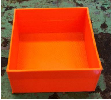
Figure 6. 50 mm x 50 mm x 25 mm 3D printed PLA frame with no infill.
