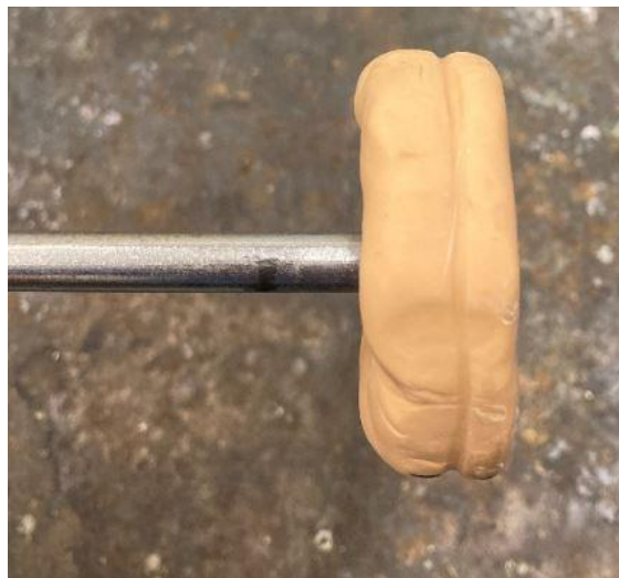
Figure 7. Side view of one clay roller with filament indentation and 9 inch bolt through its center.
