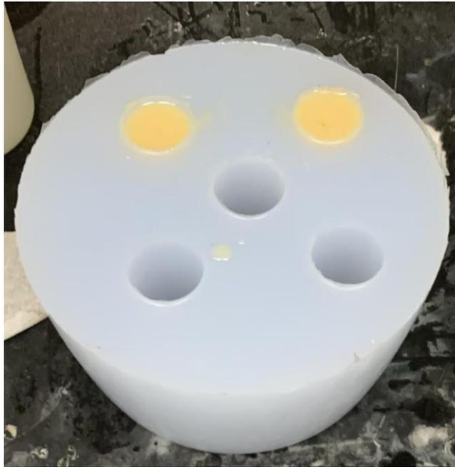
Figure 8. Silicone mold for casting cylindrical samples.
