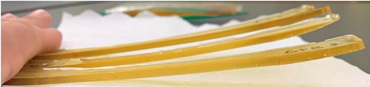
Figure 12. Tensile specimens formulated with 25wt% glass exhibit a bowed shape as a result of uneven chemical contraction during curing.
