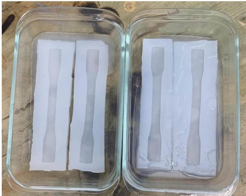
Figure 7. Silicone molds for casting tensile samples.
