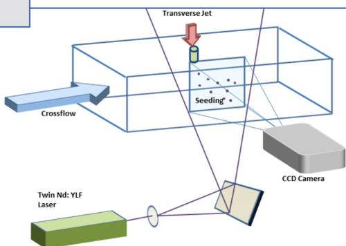
Fig 4: Schematic representation of imaging set-up for the experiment.
