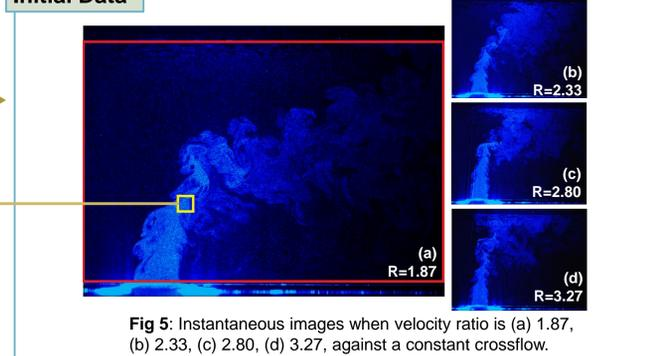
Fig 5: Instantaneous images when velocity ratio is (a) 1.87, (b) 2.33, (c) 2.80, (d) 3.27, against a constant crossflow.
