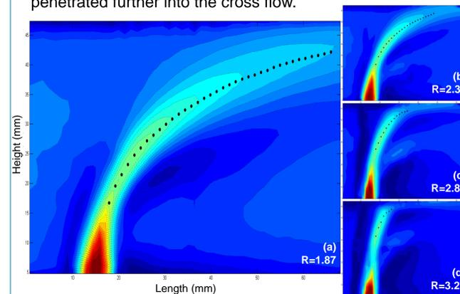
Fig 7: The vector field with a contour for the four different jet flow rates of (a) 1.87, (b) 2.33, (c) 2.80, (d) 3.27. Note that the increased jet velocity resulted in the impact against the opposite wall.
