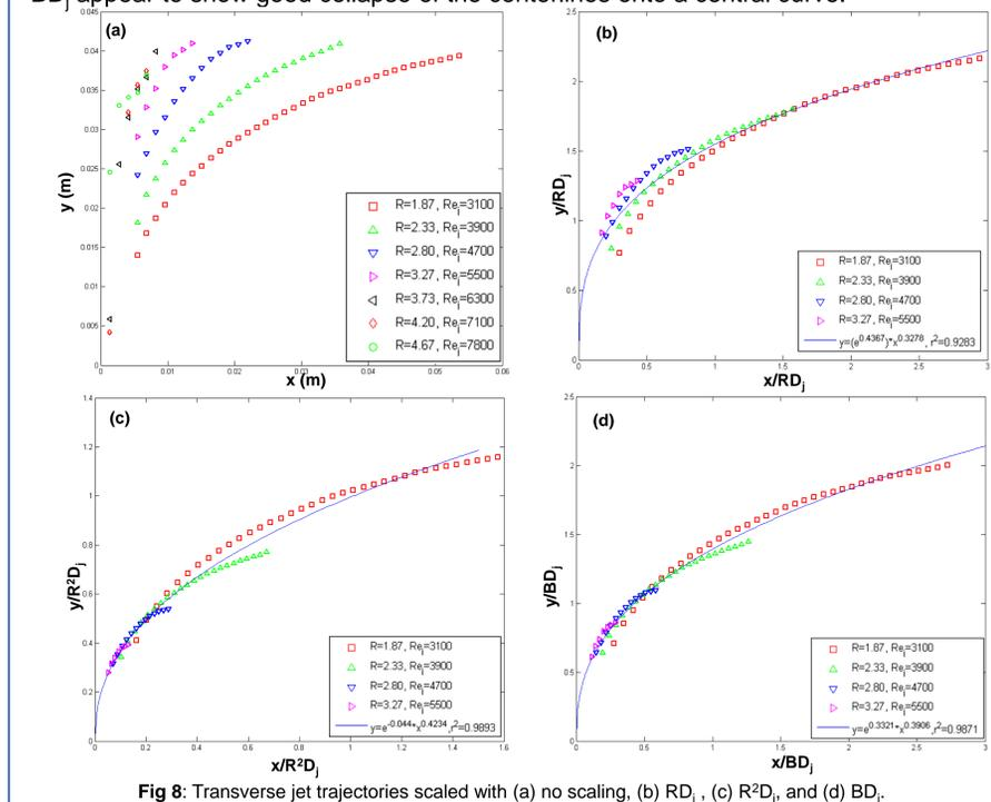
Fig 8: Transverse jet trajectories scaled with (a) no scaling, (b)  $RD_j$ , (c)  $R^2D_j$ , and (d)  $BD_j$ .
