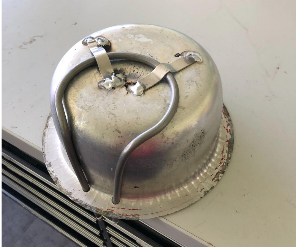
Fig. 5. Nichrome wire immersion heater bound to inner PCA pot.
