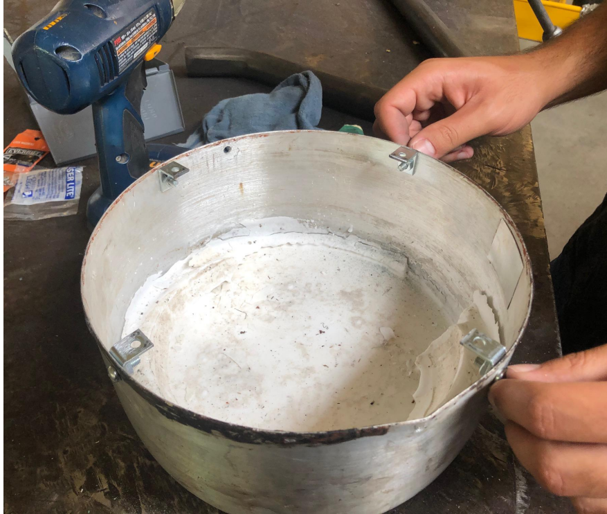
Fig. 6. Corner brackets attached to Outer PCA pot, solid solar salt shown inside
