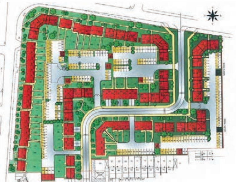
Figure 5: Plan of a Kickstart project that was evaluated with BfL and scored 1.5/20 BfL. Although the scheme was defective in many ways, this shows the large open parking areas which are notoriously insecure. (Author's archive)
