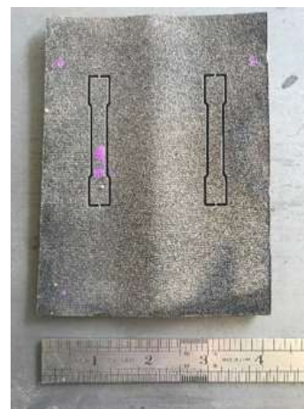
Figure 17a. As-deposited NASA-HR-1 boxes. Figure 17b. Panel cut out of Box 2 with tensile specimens cut out. A total of 24 tensile specimens were machined. The extras from the panels were used for as-built characterization.
