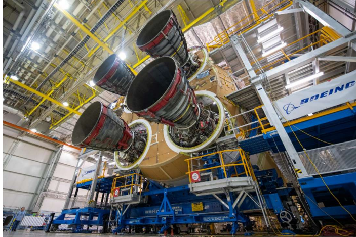
Figure 2. Four RS-25 engines secured into the SLS launch vehicle [3].
