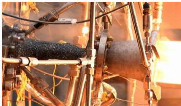
Figure 5. NASA hot fire testing of prototype DED rocket nozzle jacket [6].
