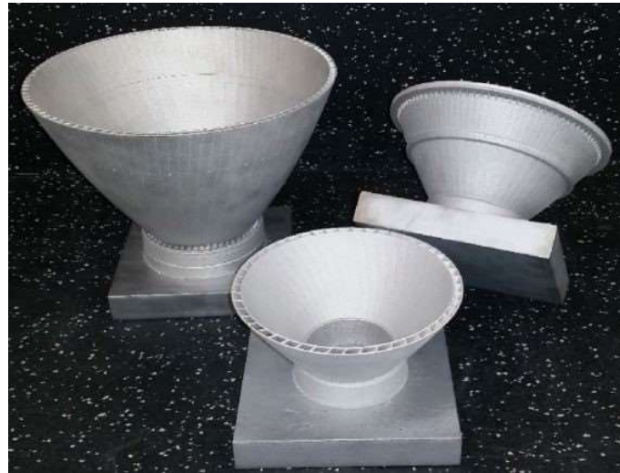
Figure 4a. Rocket nozzle schematic with separated liner and jacket. The jacket is the top component, and the liner is the vertically ribbed bottom component [7]. Figure 4b. Rocket nozzle with integrated cooling channels [6].
