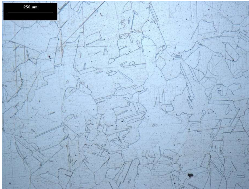
Figure 29. Heat treated JBK-75 microstructure - homogenized at 2200°F for 16 hours. 100X magnification. Etched with Kallings No. 2. Note that all homogenized samples exhibited a similar coarse-grained, equiaxed microstructure.
