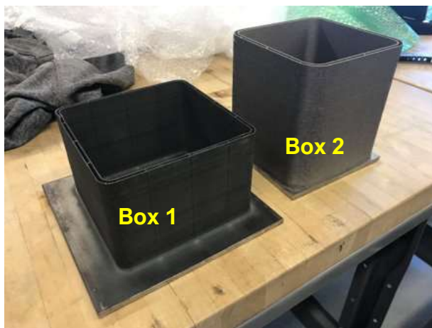
Figure 17a. As-deposited NASA-HR-1 boxes. Figure 17b. Panel cut out of Box 2 with tensile specimens cut out. A total of 24 tensile specimens were machined. The extras from the panels were used for as-built characterization.
