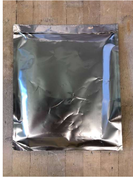
Figure 14. Stainless steel bag used to protect the NASA-HR-1 samples from oxidizing in the heat treatment furnace.
