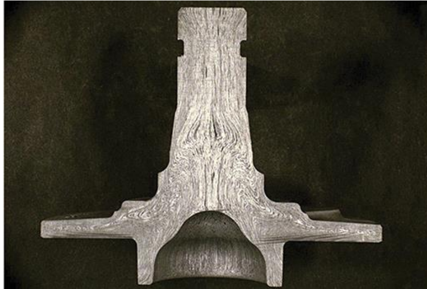
Figure 6. Cross section of a forged part that has been etched to depict grain flow [13]. The vertical lines through the longitudinal body represent the grain flow.
