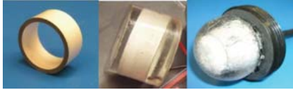
Fig. 2. From left to right: The raw piezoelectric ring ceramic, the potted ceramic, and the transducer in the potting compound mounted to a prototype plate to be attached to a modem housing.
