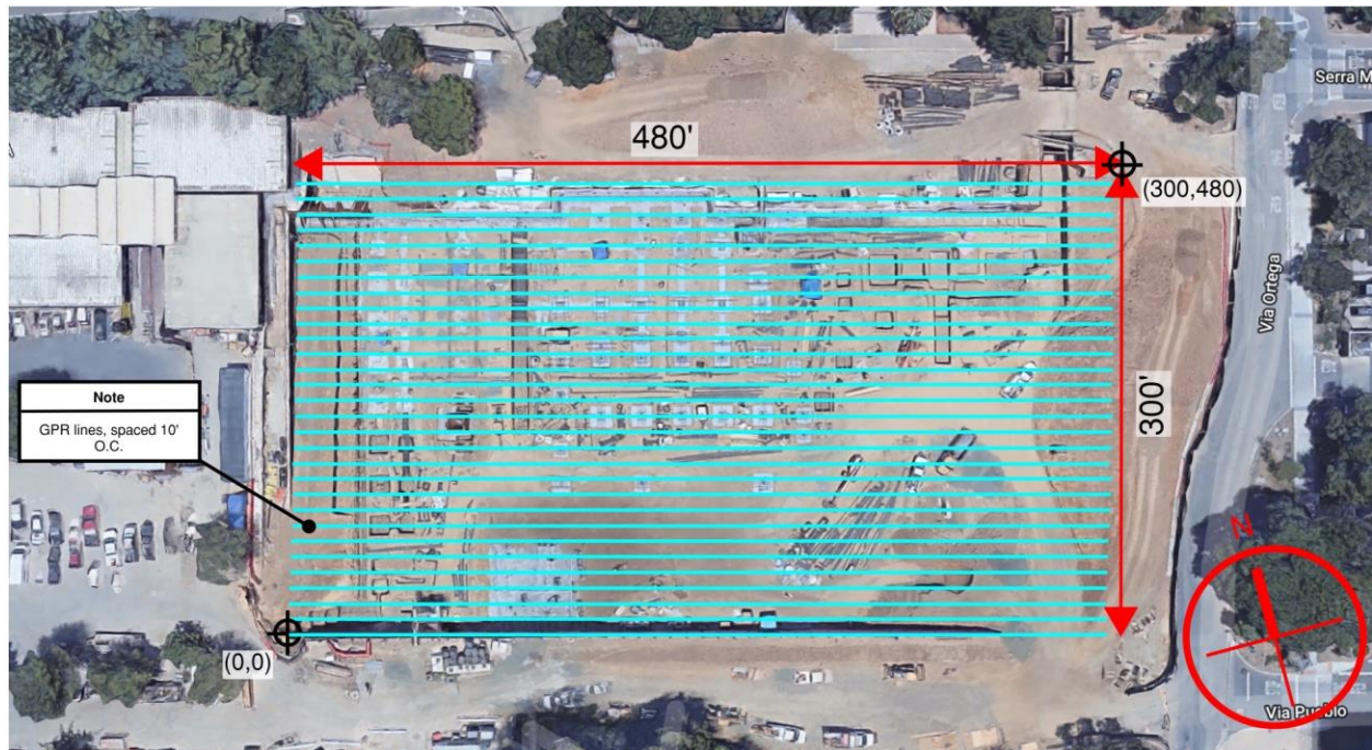
Figure 6: Representation of the survey lines used by GPR on Stanford University's ChEM-H & SNI Building
