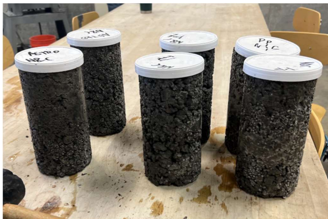
Figure 8– Preliminary Batch Cylinders at 7 Day Cure
