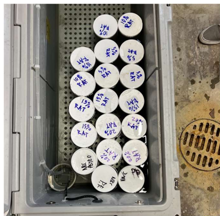
Figure 10- Proportion Batch Placed in Temperature Regulated Subaquatic Curing Chamber
