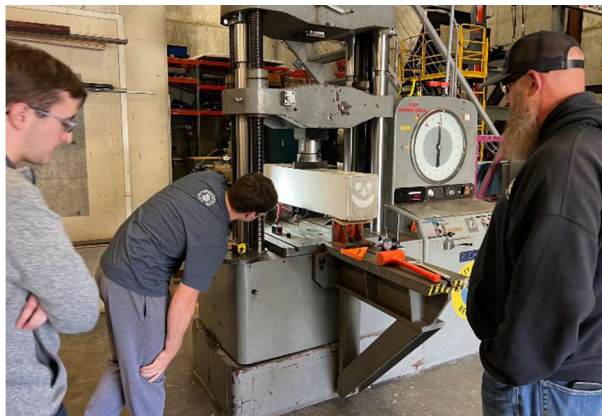
Figure 22 - First Beam in Mechanical Press
