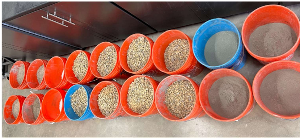
Figure 11– First and Second Beam Measured Concrete Mixes
