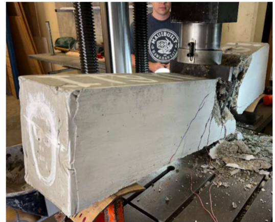
Figure 36 - Second Beam Failure at 30.00 kips
