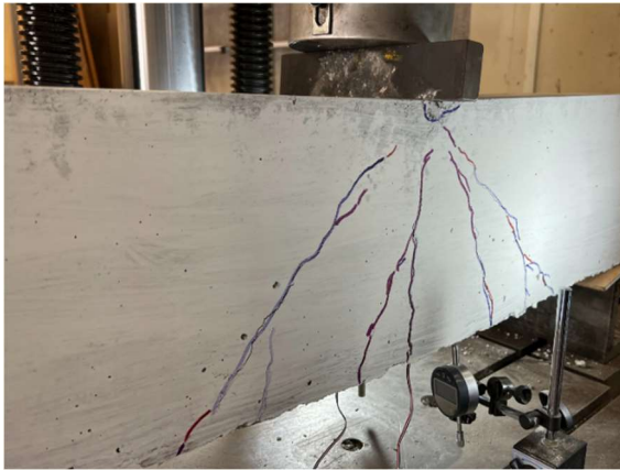
Figure 35 - Second Beam Crack at 24.03 kips
