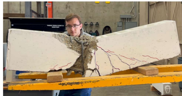
Figure 23 - First Beam Failure on Forklift
