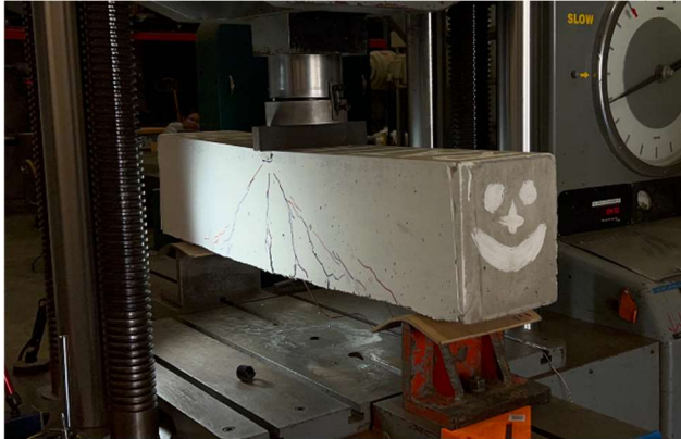
Figure 33 - First Beam Cracks 28.52 kips
