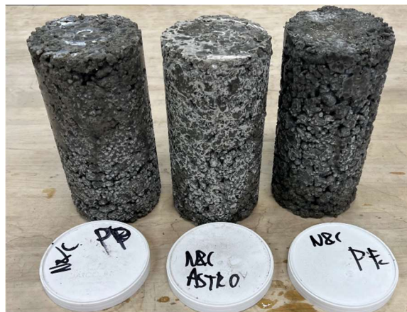
Figure 9 - Preliminary Batch Cylinders at 28 Day Cure
