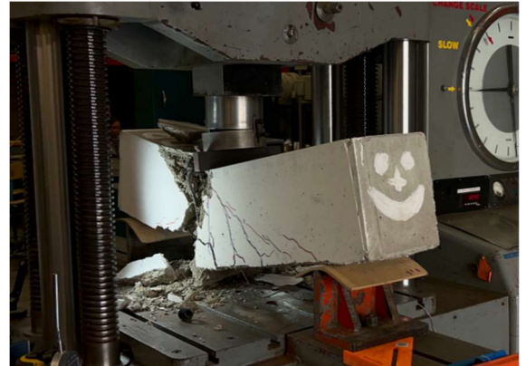
Figure 34 - First Beam Failure at 36.50 kips
