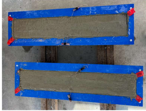
Figure 17 - Poured Beams with Removed Caged Supports
