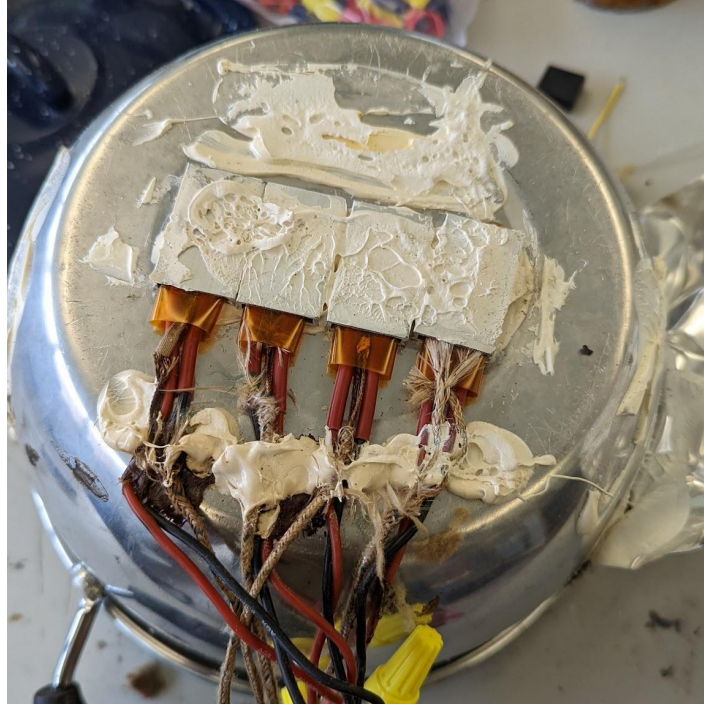
Fig. 13 shows the PTCs connected to a shunt resistor by use of an electrical nut, and the thermocouples are on the inside center of the PTC.
