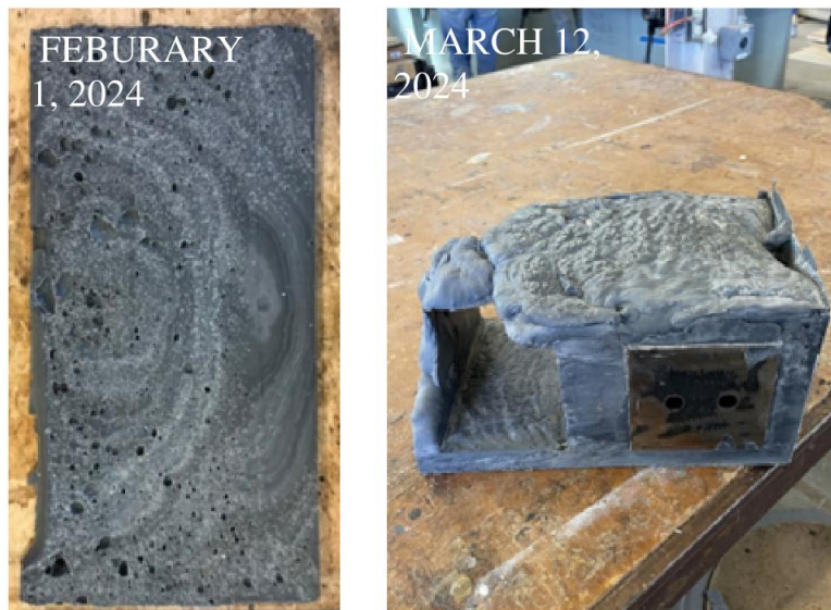
Figure 1 Porous Extrusion (left), Partially Extruded Brick (right)
