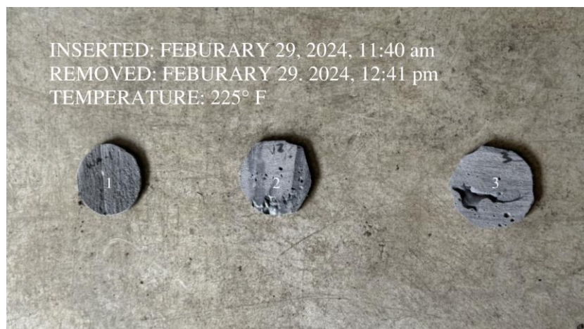
Figure 1010 ASTM-D570 Conditioned Specimen
