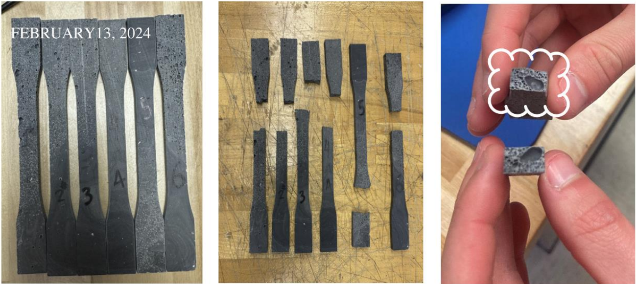
Figure 9 Test samples before (left) and after (middle) test. Air bubble occurring at failure (right)
