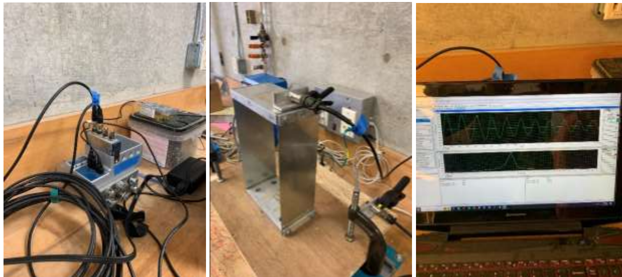
Figure 21. Instrumentation: (a) Accelerometers, (b) NI CompactDAQ, (c) Laptop
