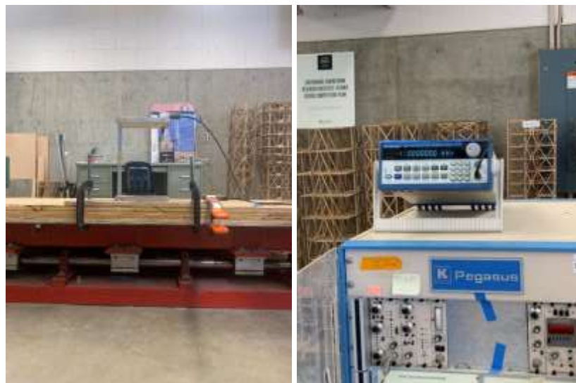
Figure 20. Uni-Directional Shake Table: (a) Platen, (b) Control Panel
