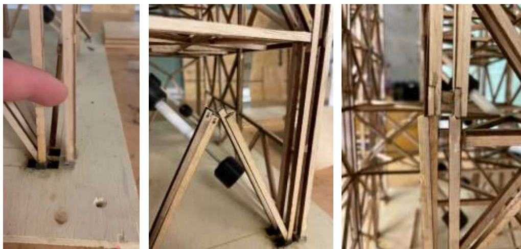
Figure 26. Competition Building Model Issues: (a) Insufficient Penetration Depth for Base Columns, (b) Load Redistribution Resulted in Brace Failure, (c) Column Splices Not Staggered
