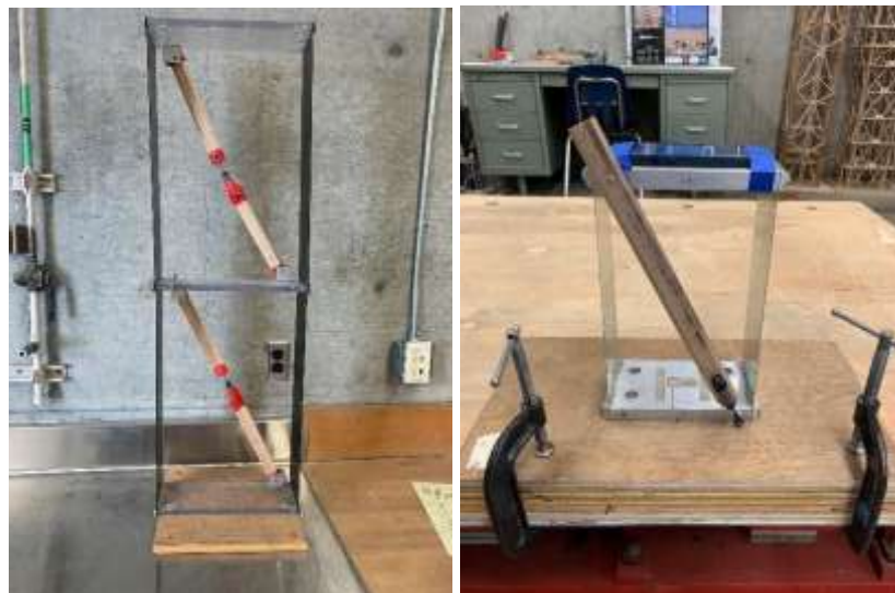
Figure 19. Damper Test Specimen: (a) MDOF Model, (b) SDOF Model
