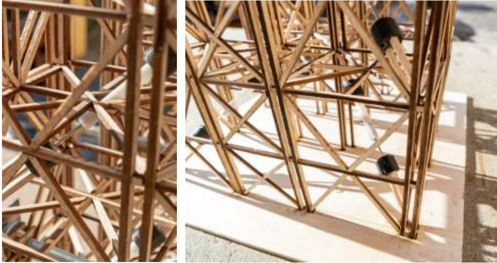
Figure 18. Final Competition Model Details: (a) Damper through Diaphragm Penetration, (b) Brace-to-Column Connection
