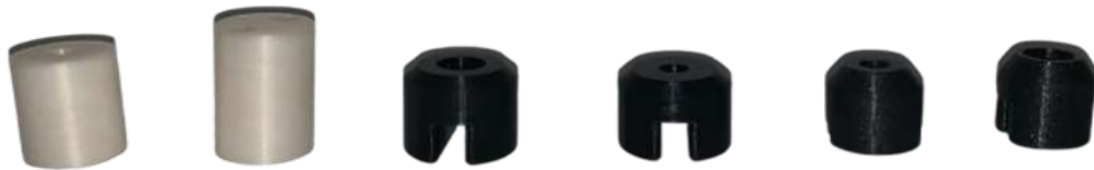
Figure 11. 3-D Printed Damper Connection Caps: Iterations 1, 2/3, and 4 (left to right)
