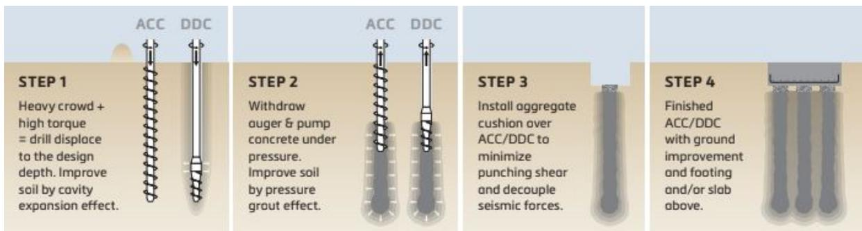
Figure 2: 4-Step Construction Process
