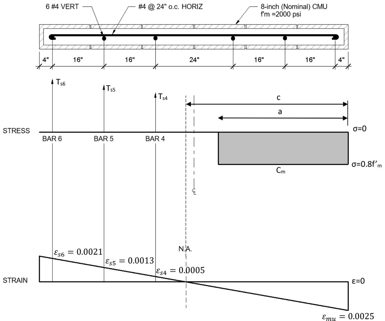
Figure 3.6: Stress and Strain diagrams labeled with the appropriate force resultants and strain values at the balanced condition.
