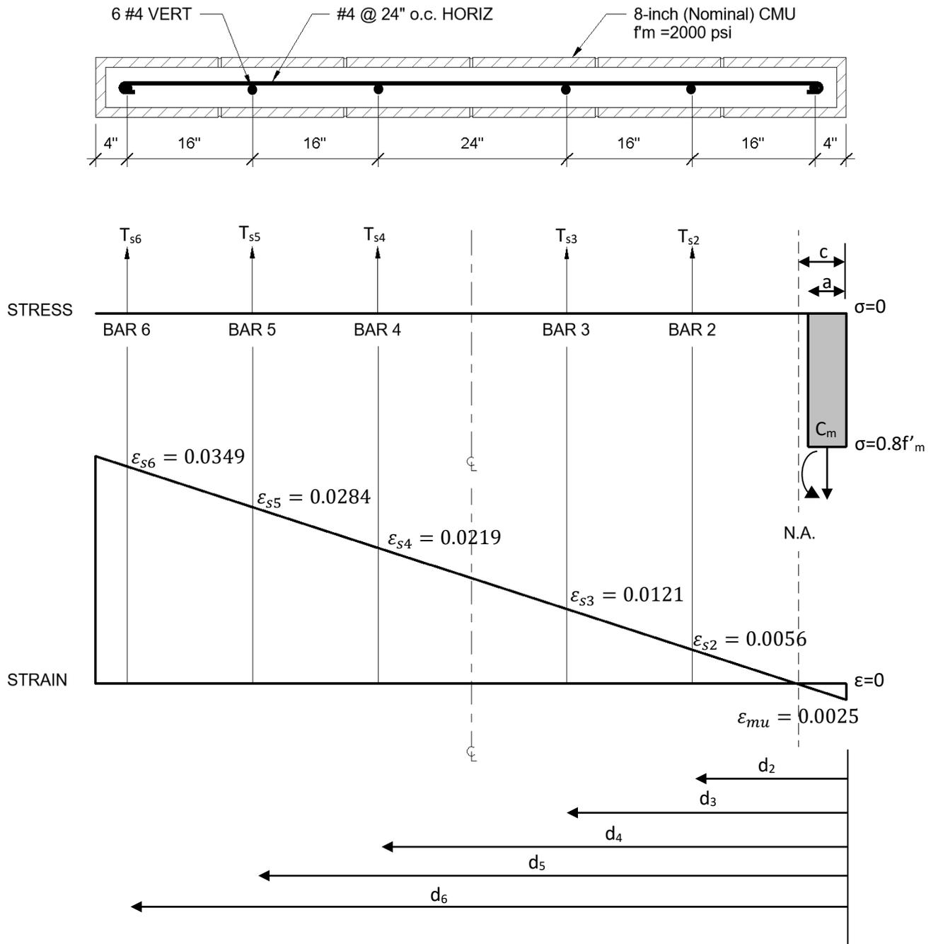
Figure 3.5: Stress and Strain diagrams labeled with the appropriate force resultants and strain values at the pure flexural condition
