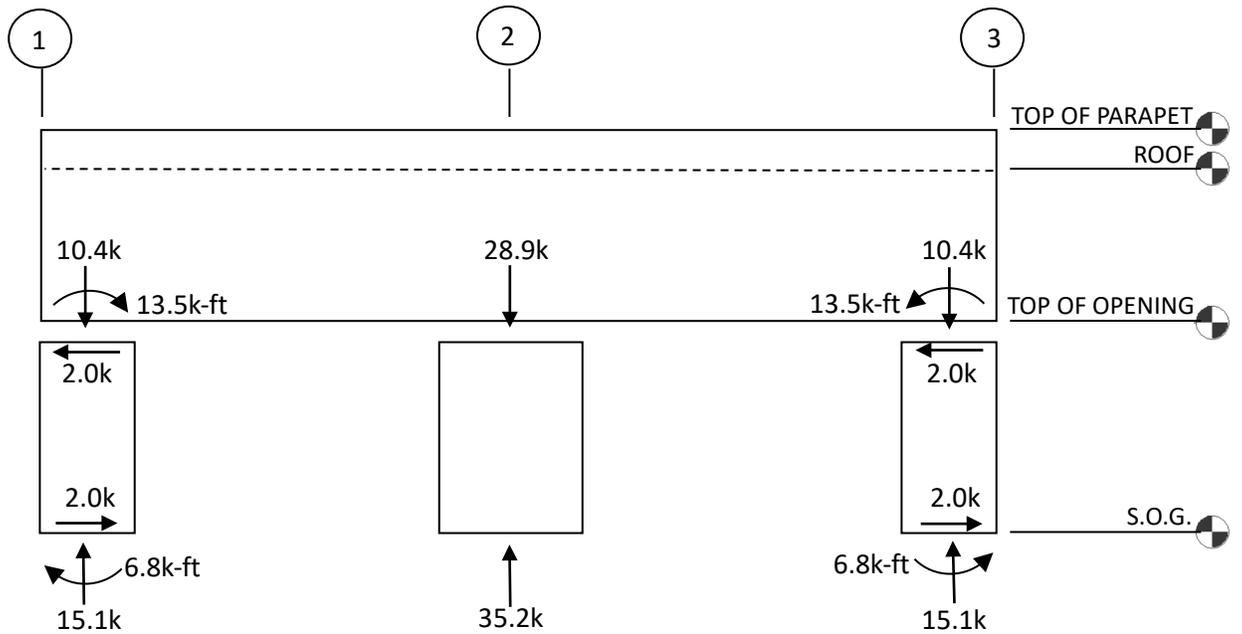
Figure 3.3: Dead loads along the wall-line
