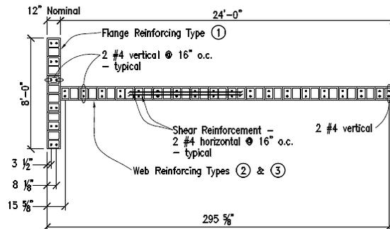
Example Shear Wall - Plan and Reinforcing
