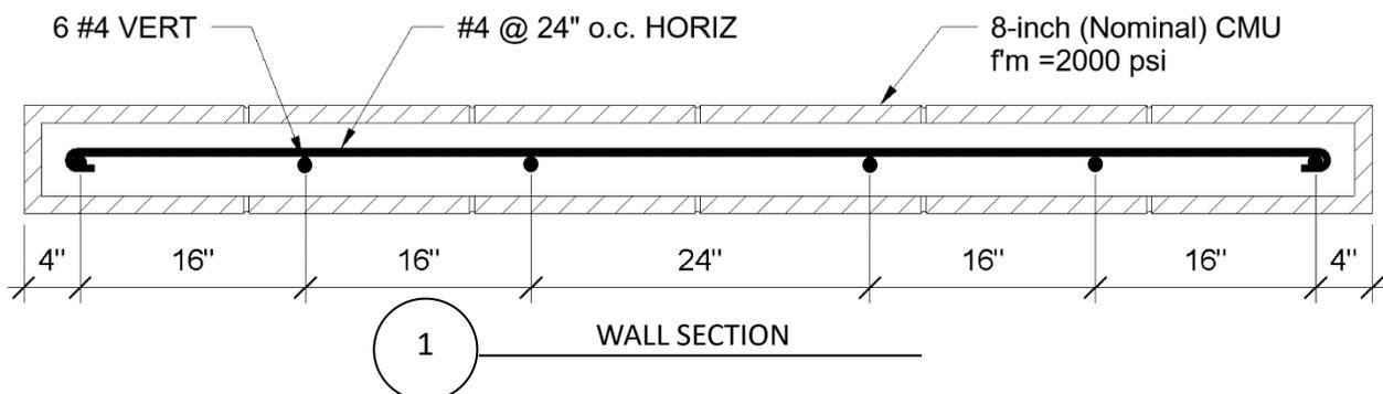
Figure 3.2: A section cut through the wall segment being analyzed that shows the reinforcement spacing.
