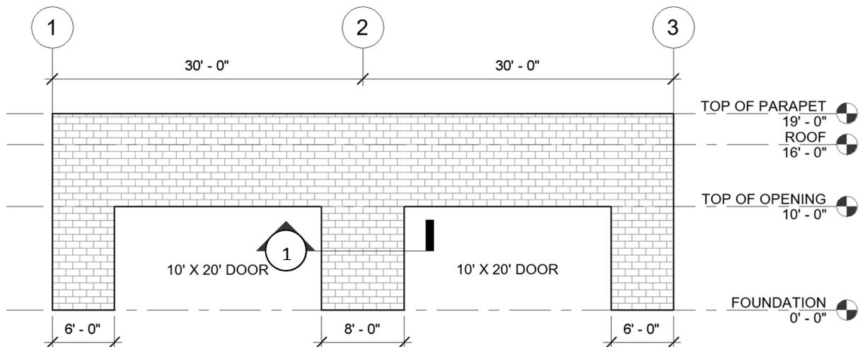
Figure 3.1: An elevation of the wall with a section cut through the wall being analyzed.
