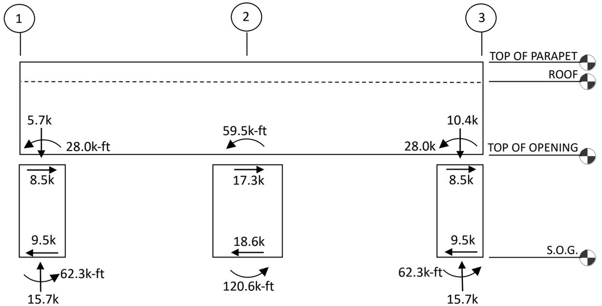
Figure 3.4: Earthquake loads along the wall-line
