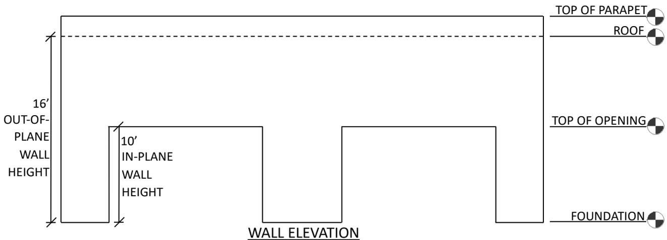
Figure 4.1: Wall elevation depicting both in-plane and out-of-plane heights
