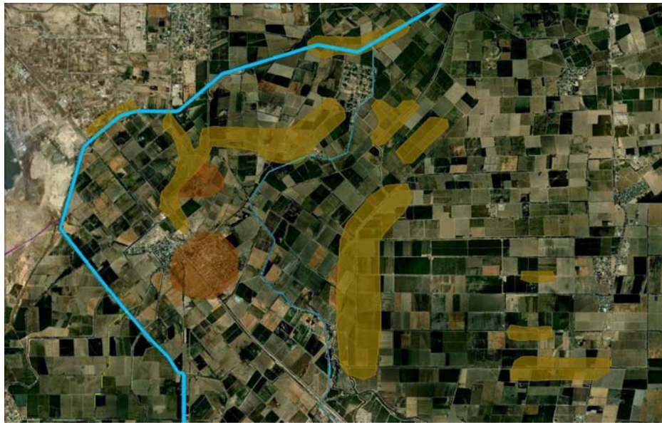
Figure 4. Zones of liquefaction in relation to the Reforma Canal and Nuevo Delta Canal.
