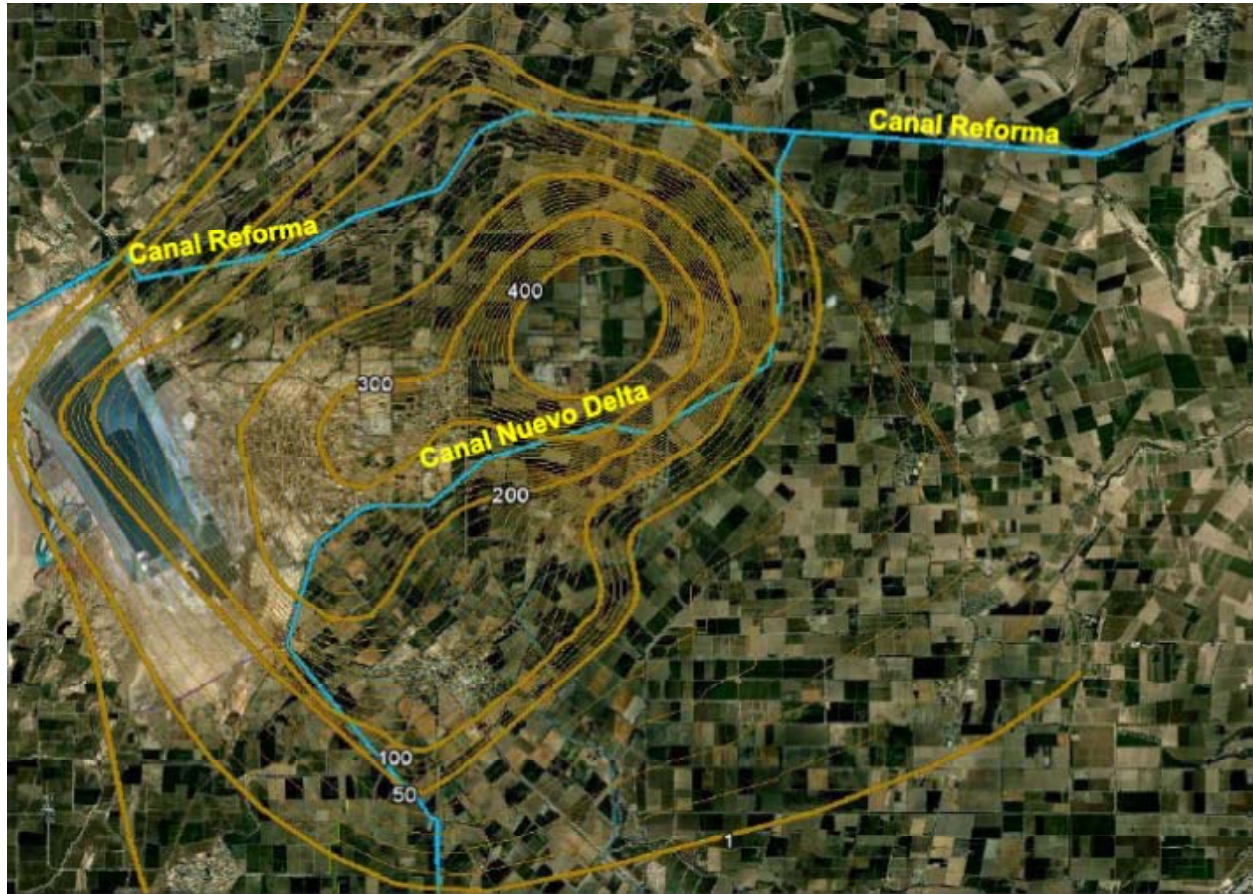
Figure 2. Lines of equal subsidence predicted by CICESE to occur within 30 years. Units are cm. The geothermal production zone is on the center left-hand side of the figure. The blue lines show the Reforma Canal (top, flowing right to left), and the old, damaged Nuevo Delta Canal (center, flowing from top to down).
