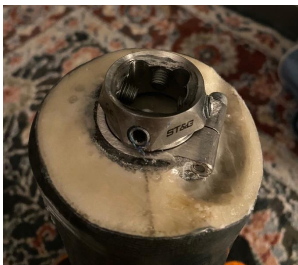
Figure 15: Modular stem attachment point for a prosthetic foot from Mr. Bolin's most recent leg. Screws will be inserted into the 4 tapped holes as seen in the figure.
