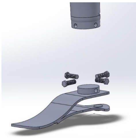
Figure 11. Exploded view of shell-foot interface. The interface between the shell and the foot will be held in place by 4 screws.
