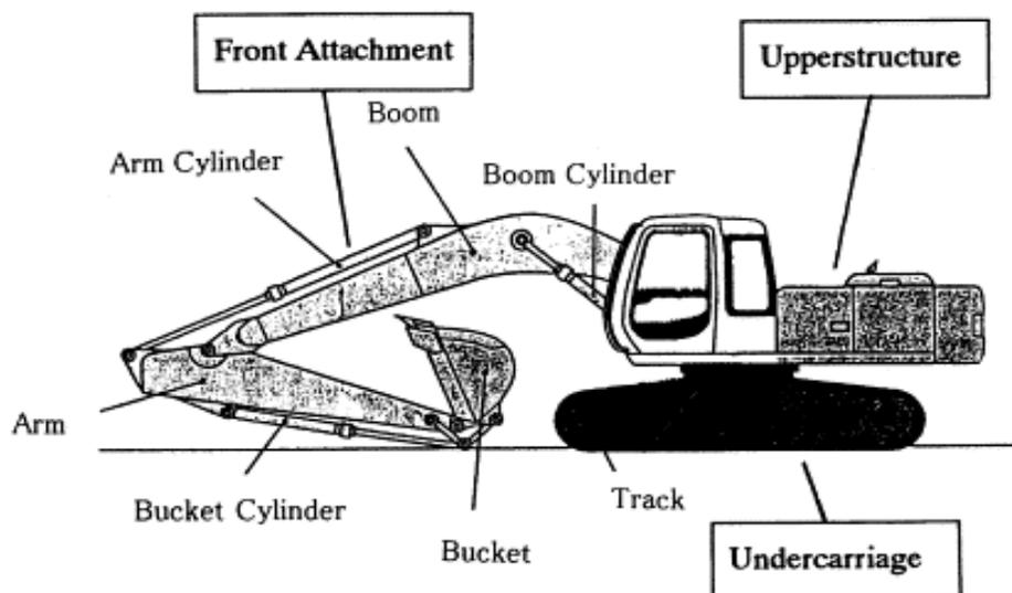
*Figure 1-Hydraulic Excavator Constitution*
