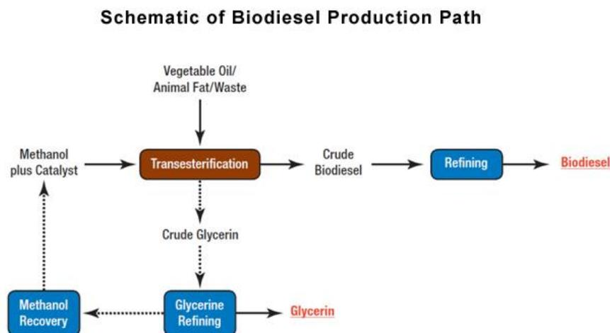
Figure 2-Biodiesel Production and Distribution
