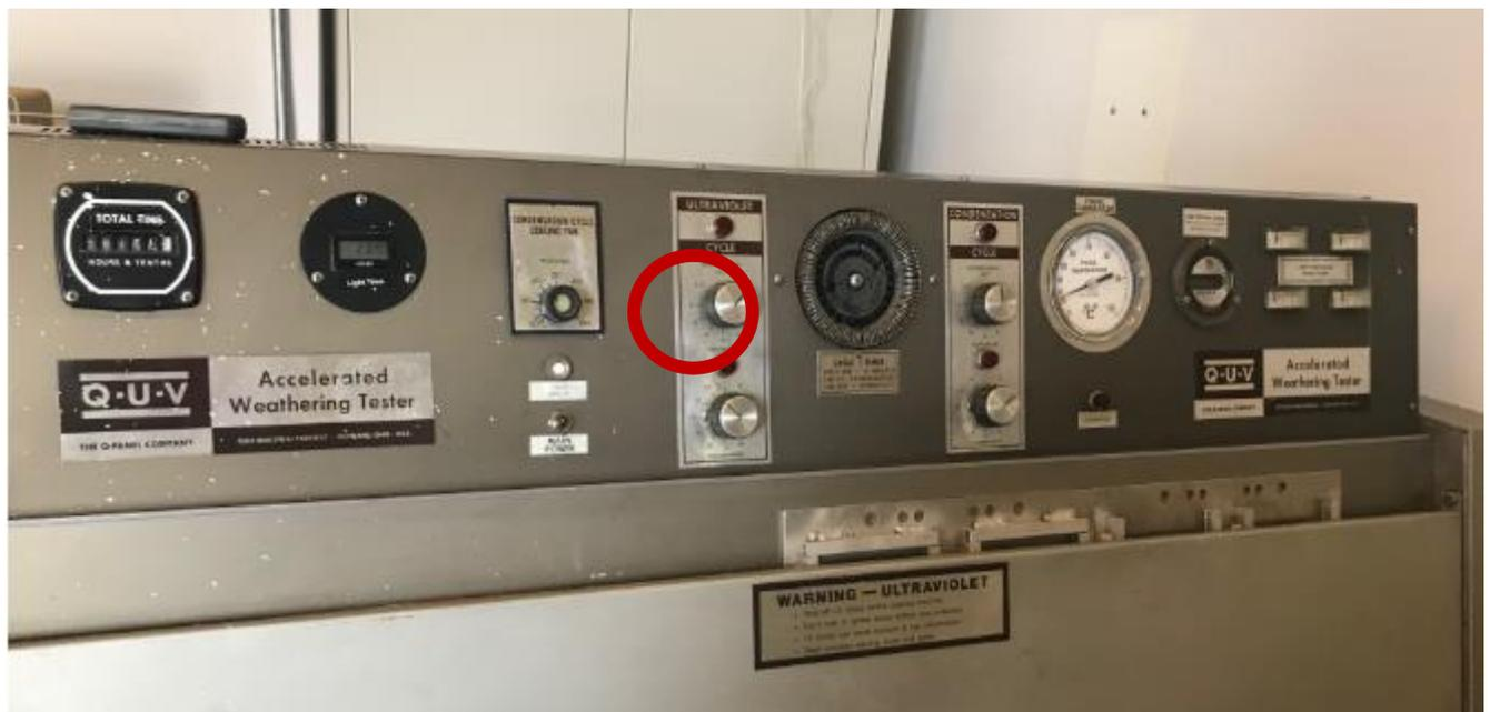
Figure 4. Q-U-V Accelerated Weather tested with the heater know highlighted.
