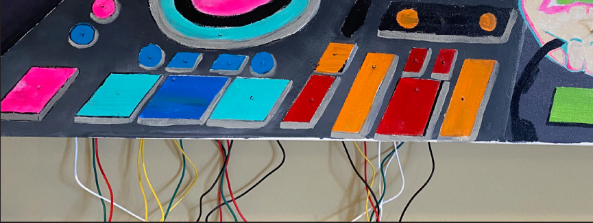
Front of Painting; Conductive paint recolored with nails through the center.
