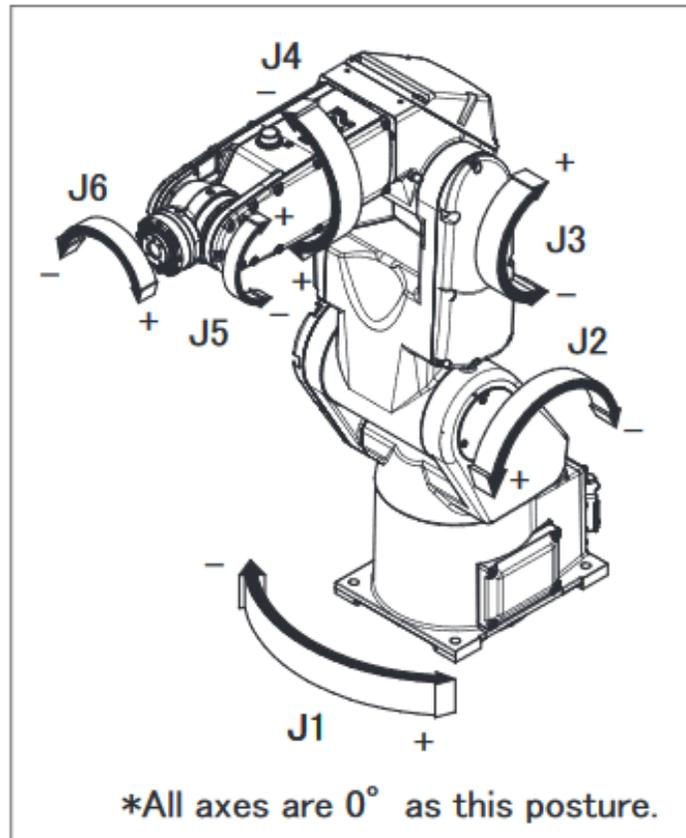
**Figure 4:** Robot Joints
