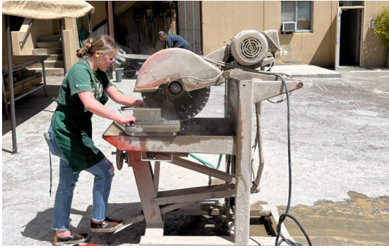
Figure 9. Wet saw used to cut grout samples out of CMU cells
