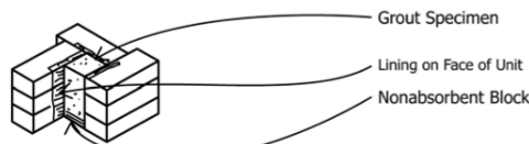
FIG. 1 Example of Grout Mold (Units 6 in. (152.4 mm) or Less in Height, \frac{2}{4} in. (57.2 mm) High Brick Shown)
