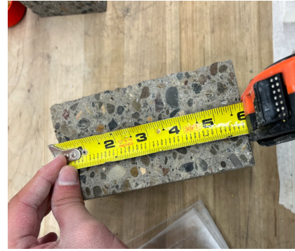
Figure 10. Sample height measured at mid-height
