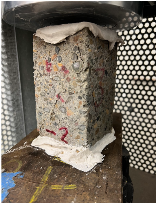
Figure 15. Sample failure following compression test
