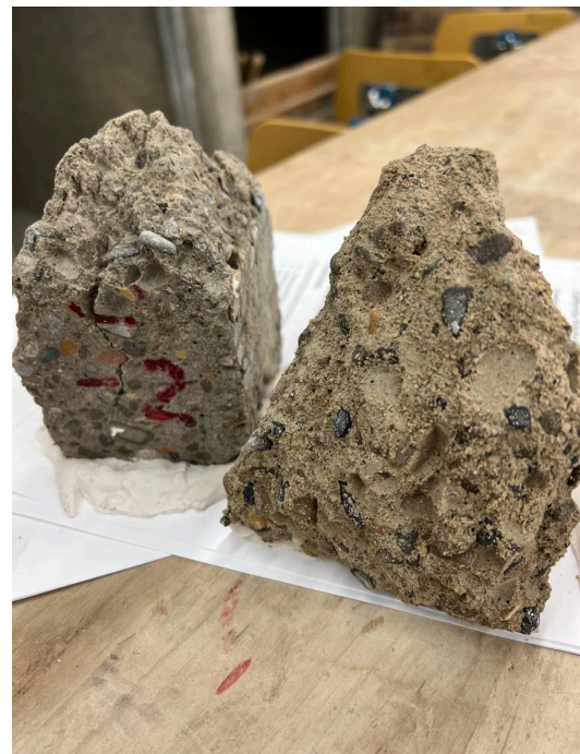
Figure 14. Tan coloring of sample containing excessive sand
