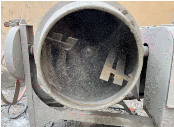
Figure 3. Mixing with electric concrete mixer
