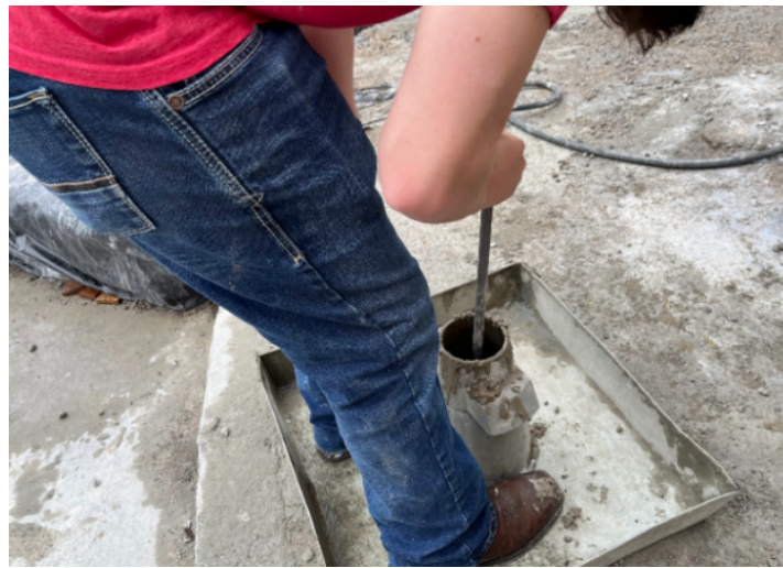
Figure 6. Rodding grout with correct foot placement
