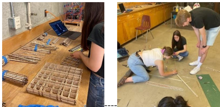
Figure 7.1. (a) Completed Diaphragms (b) Students Splicing Continuous Column Members
