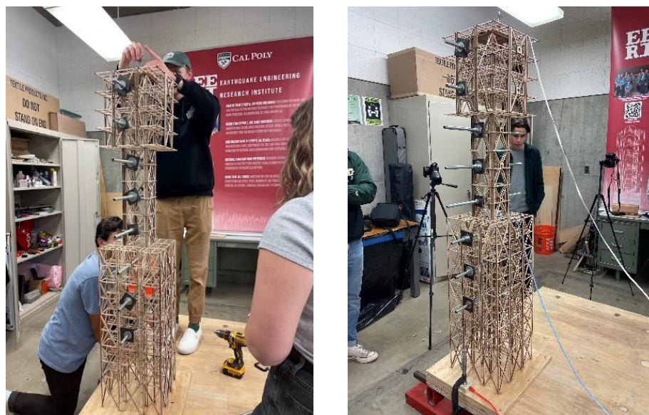
Figure 8.4. (a) Loading Structure with Threaded Rods (b) Accelerometer Locations
