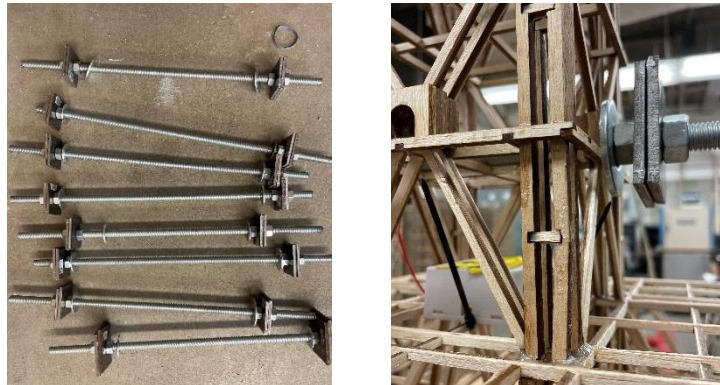
Figure 8.1. Threaded Rods with Dead-Load Weights
