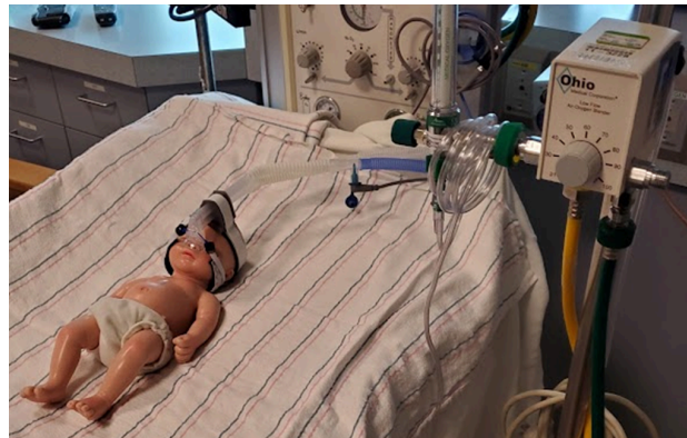
Figure 13. Model baby connected to BCPAP machine using our final prototype interface
