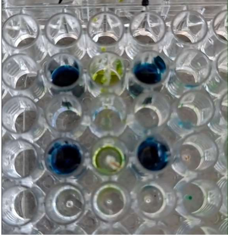
Figure 38. Example of device after 24 hours of simulated incubation. Blue represents media. Yellow represents Matrigel.
