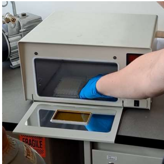
Figure 37. Loading platforms into the crosslinker
