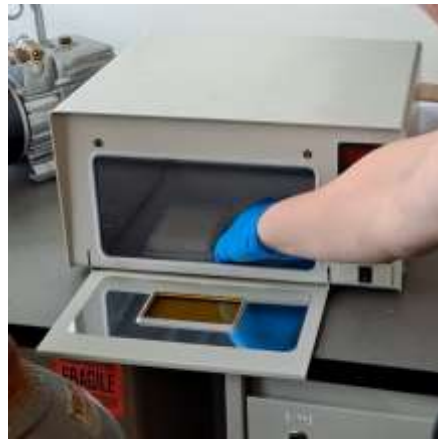
Figure 27. Loading platform in crosslinker.
